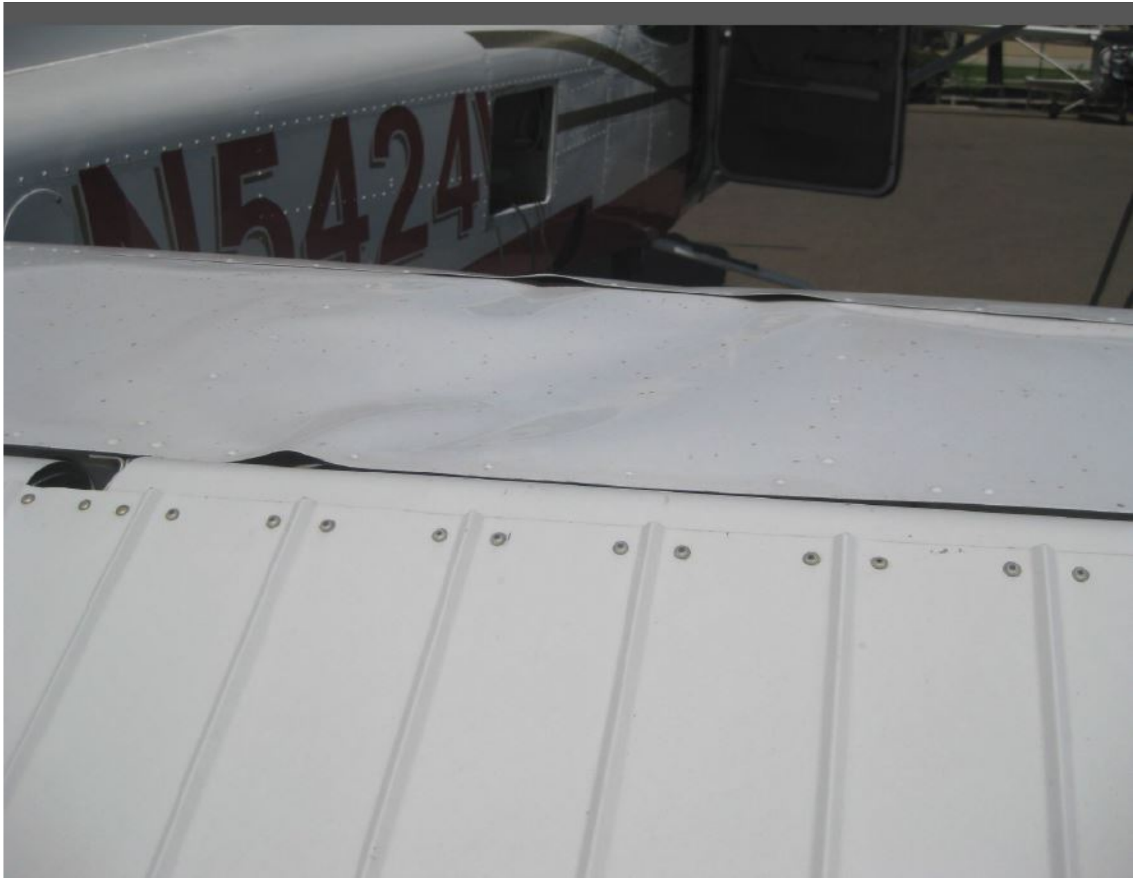
Photo 1 – Substantially Damaged Right Elevator (Photo Courtesy of FAA)
