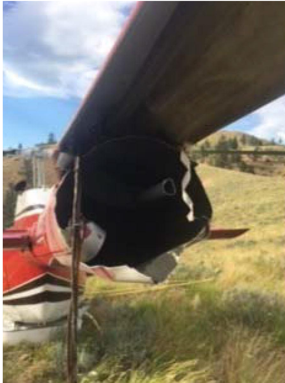
Photo 1 – View of tail boom damage (photo courtesy of the FAA)
