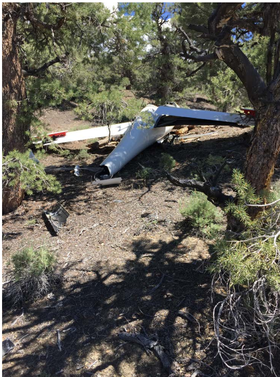
Photo 1 – Substantially Damaged Fuselage and Wings (Photo Courtesy of Operator)
