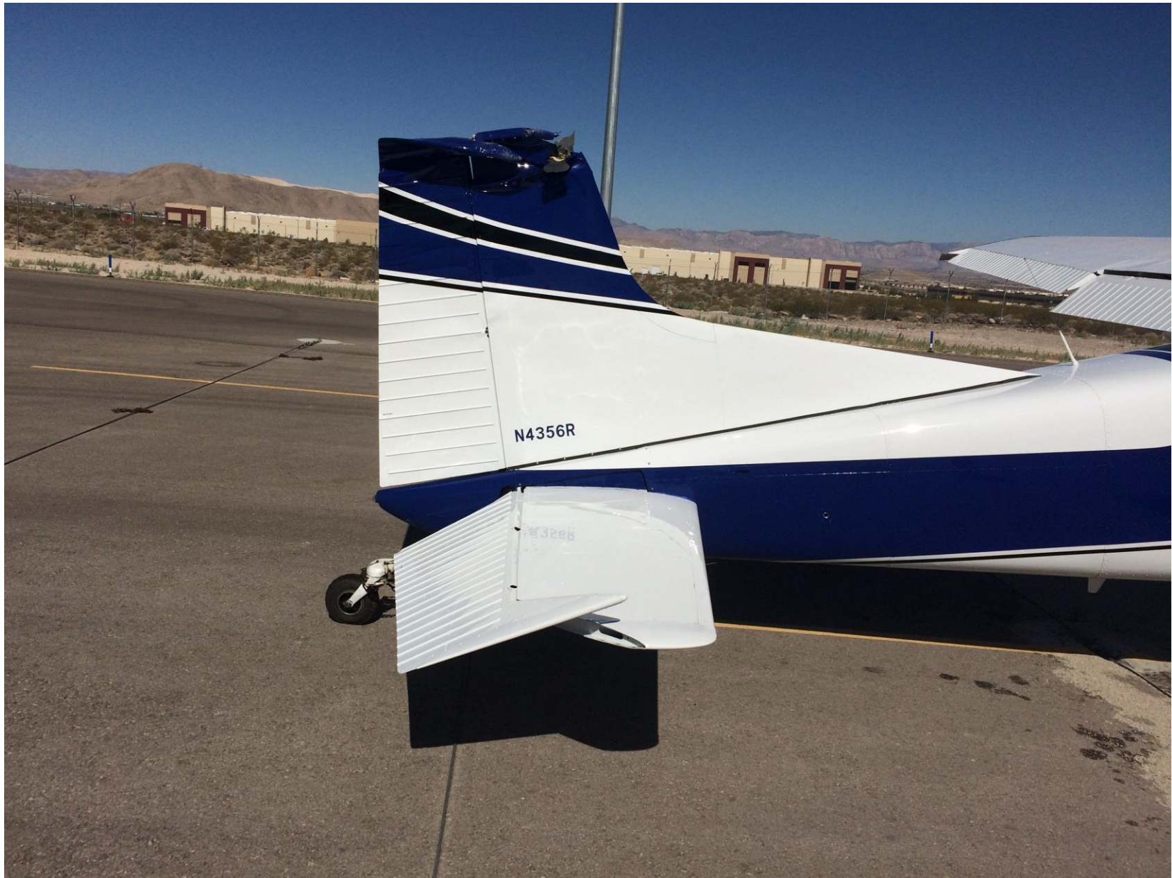
Photo 1 – View of damaged vertical and rudder (Photo courtesy of the FAA)
