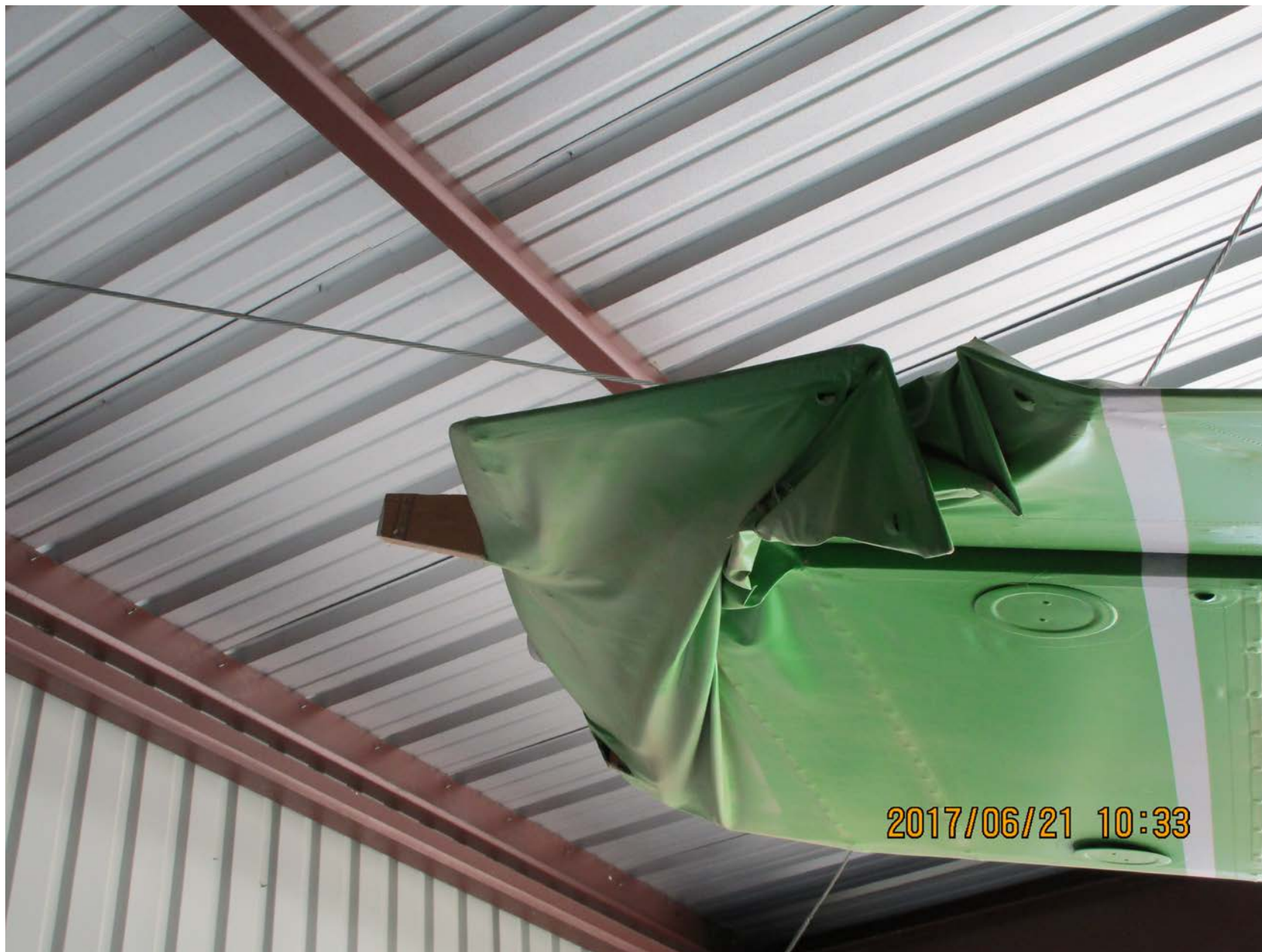
Photo 2 - Substantially Damaged Aileron and Left Wing (Photo Courtesy of FAA)
