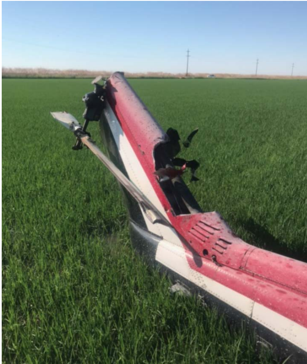
Photo 1 – View of damaged tailboom (photo courtesy unknown)
