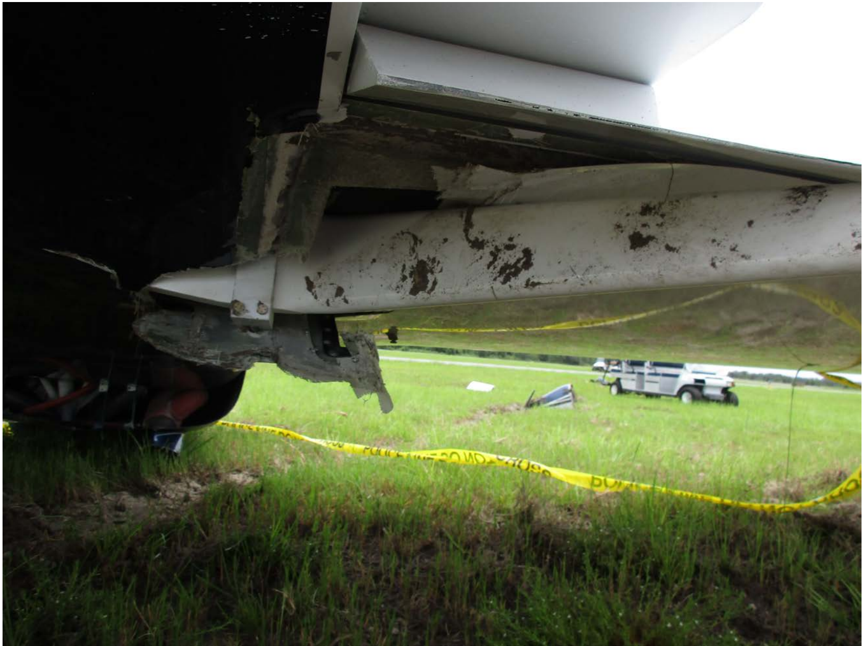
Photo 1 – View of the damage to the composite lower fuselage (Courtesy of FAA)
