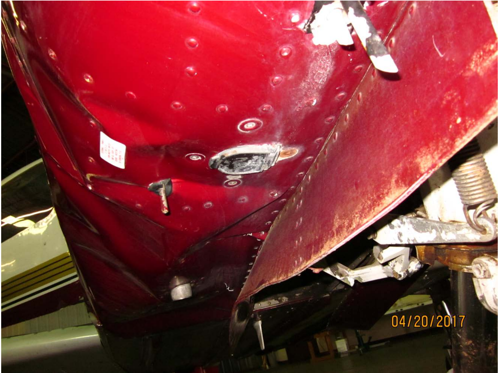
Photo 1 – View of damaged nose gear support structure (photo courtesy of the FAA)
