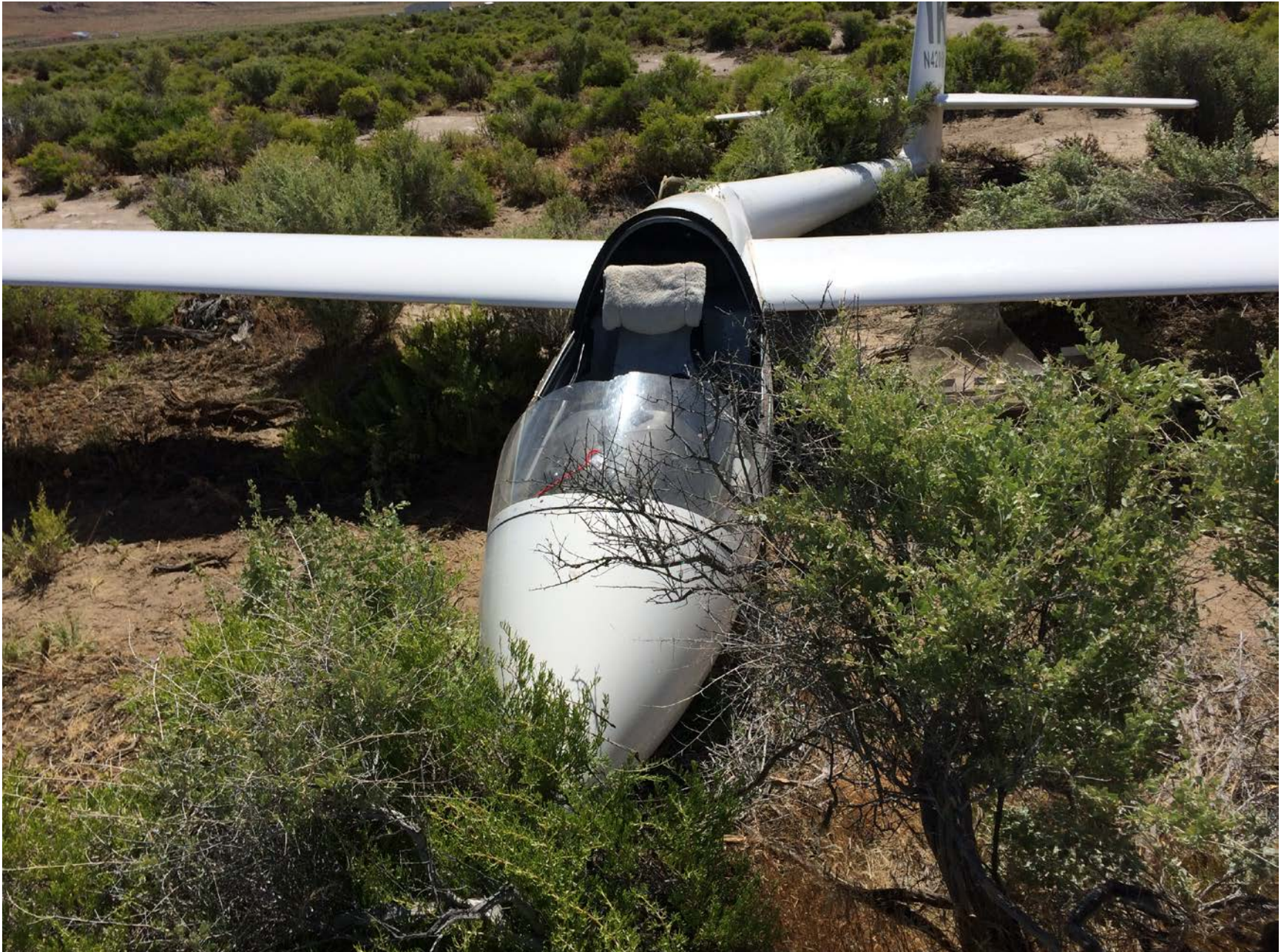
Photo 1 – View of damaged fuselage from front (photo courtesy of the FAA)
