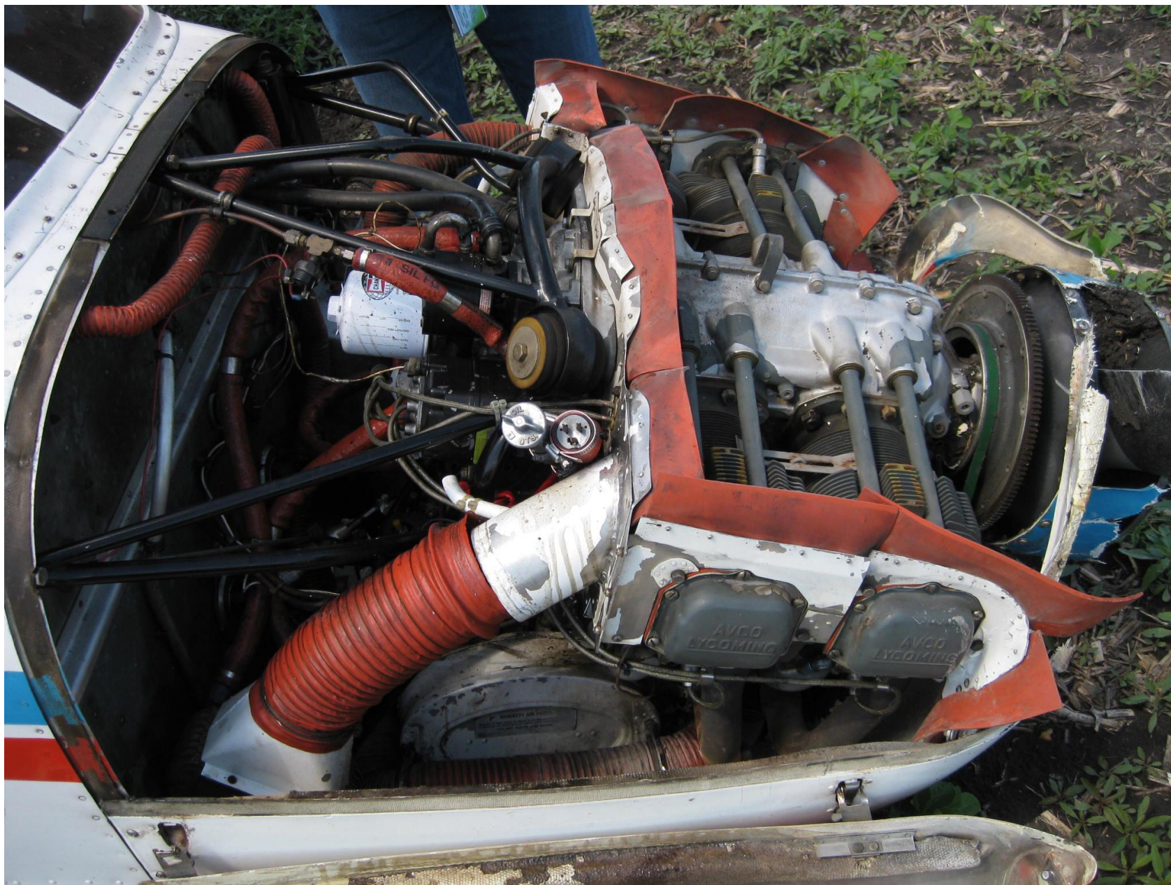
Photo 2 - View of broken engine mount (photo courtesy of the FAA)
