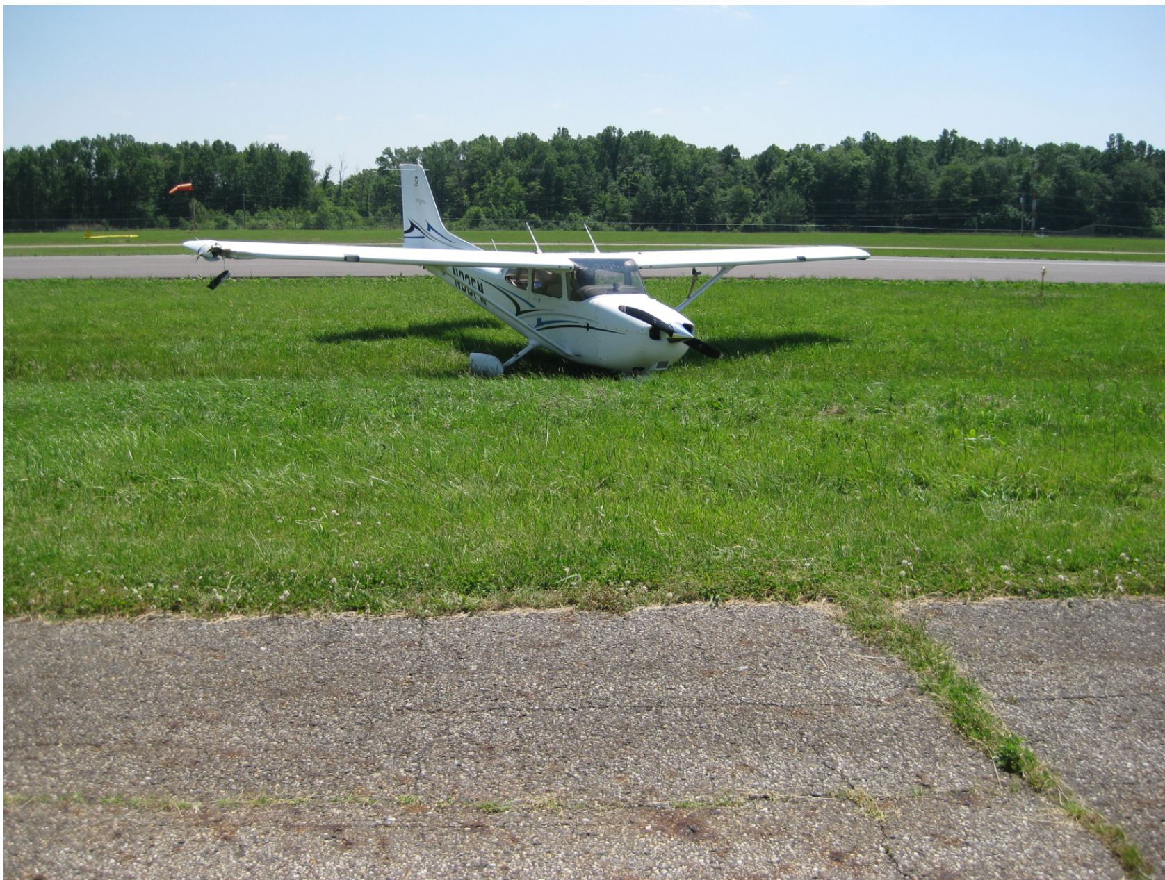
Photo 1 – View of Airplane off Runway with Collapsed Nose Gear (Photo Courtesy of FAA)
