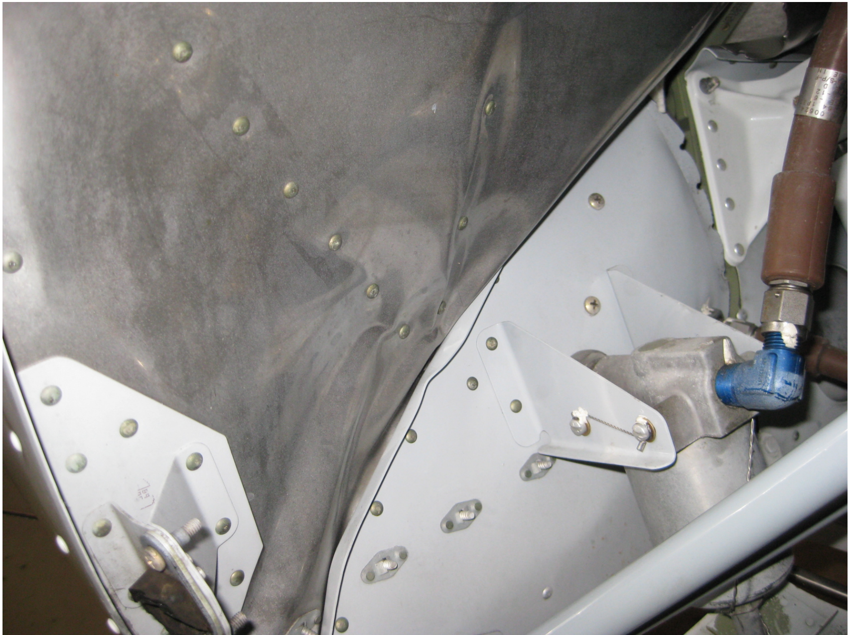
Photo 2 – Substantially Damaged Firewall (Photo Courtesy of FAA)
