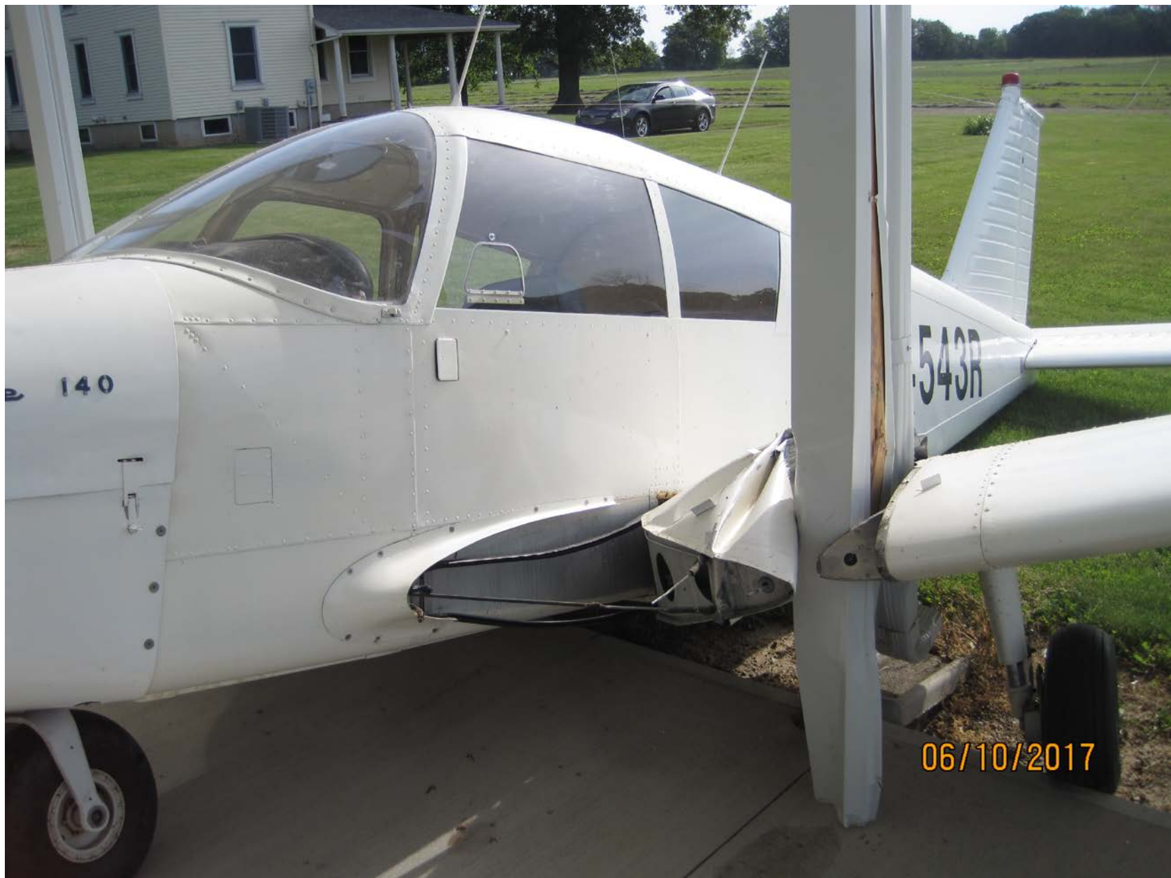
Photo 2 – View of damage to the left wing (Courtesy of FAA)
