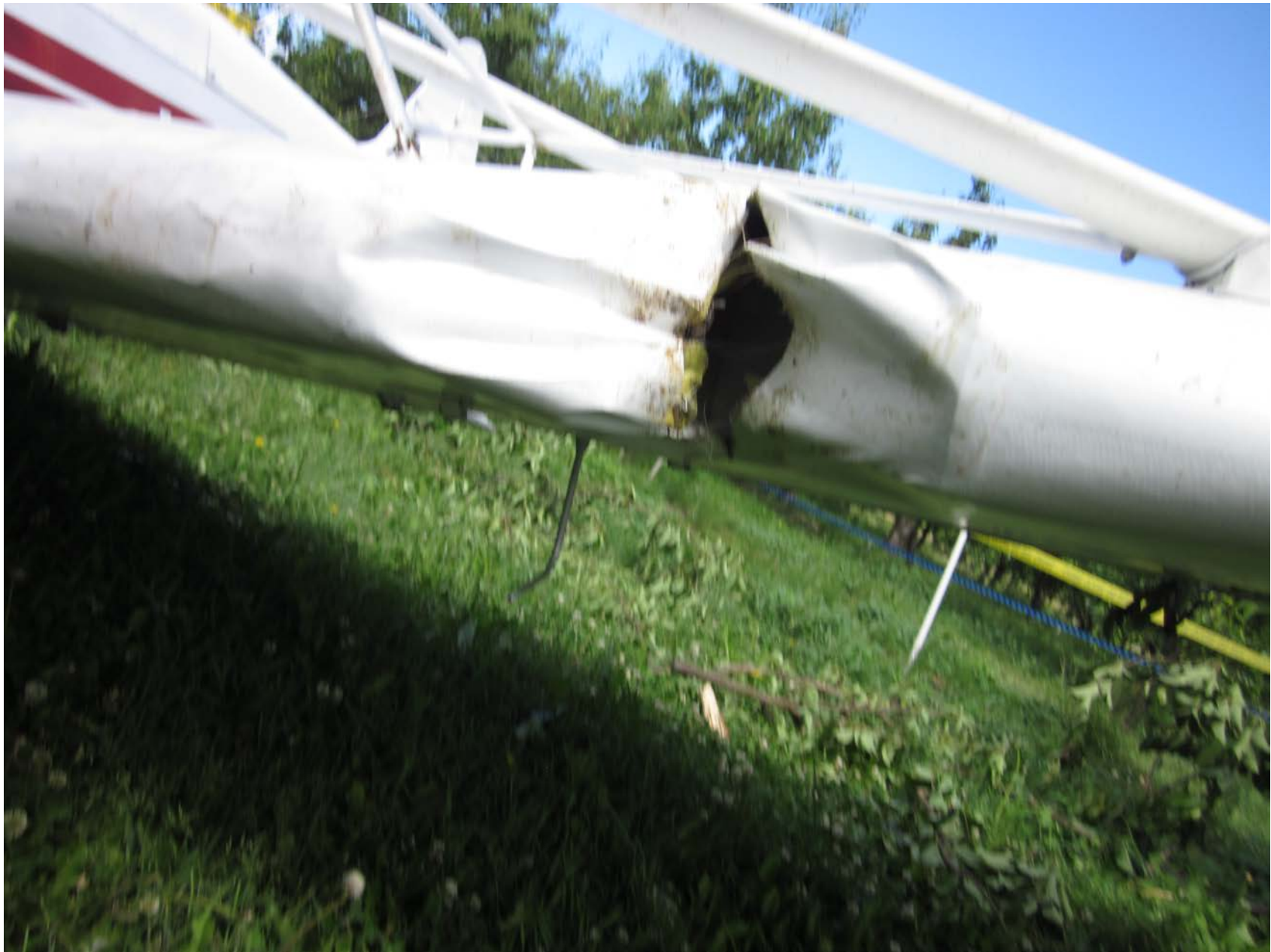
Photo 2 – View of Left Wing Spar Damage (Photo Courtesy of FAA)
