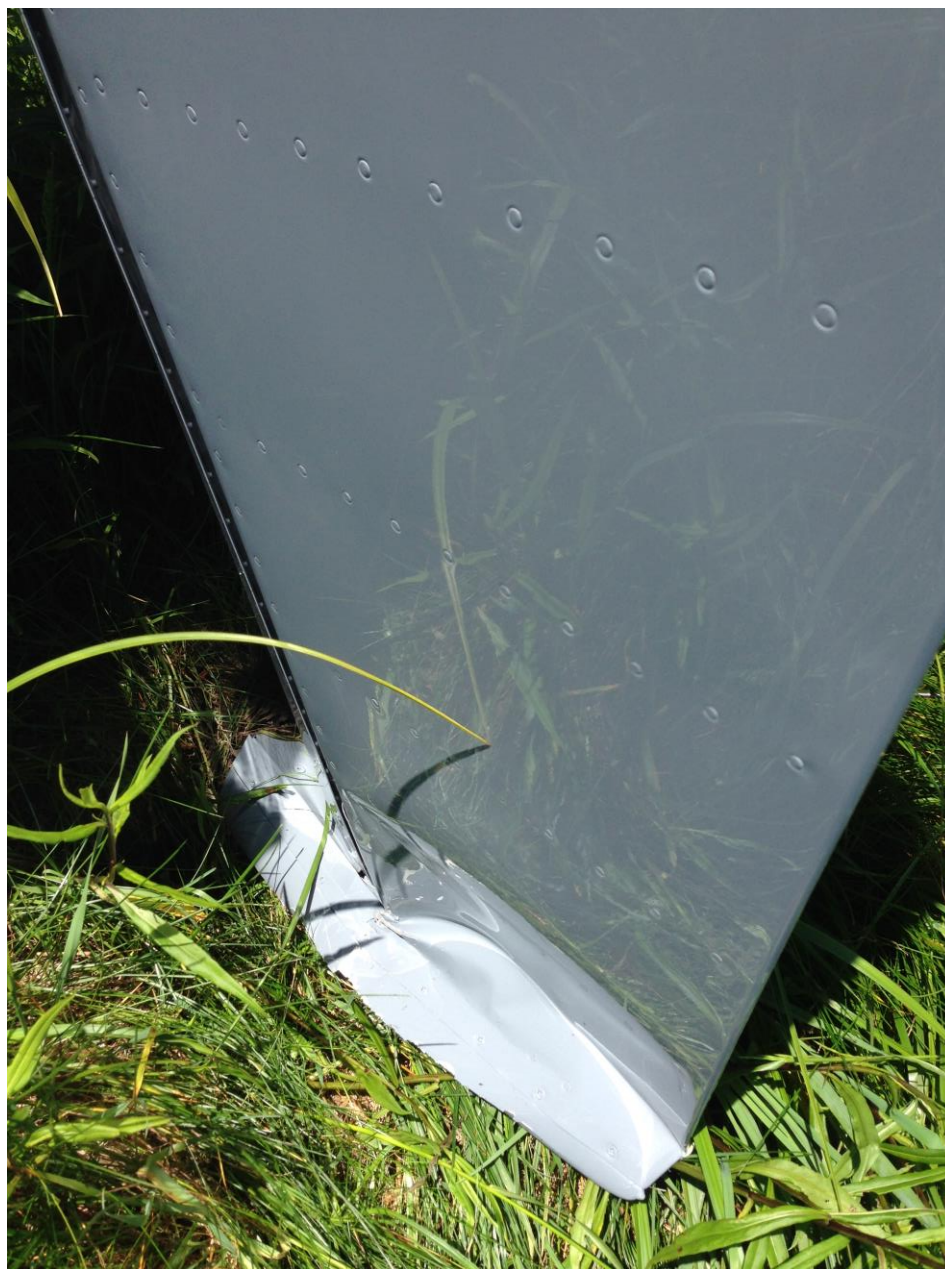
Photo 1 – View of inverted damaged rudder (Photo courtesy of the FAA)
