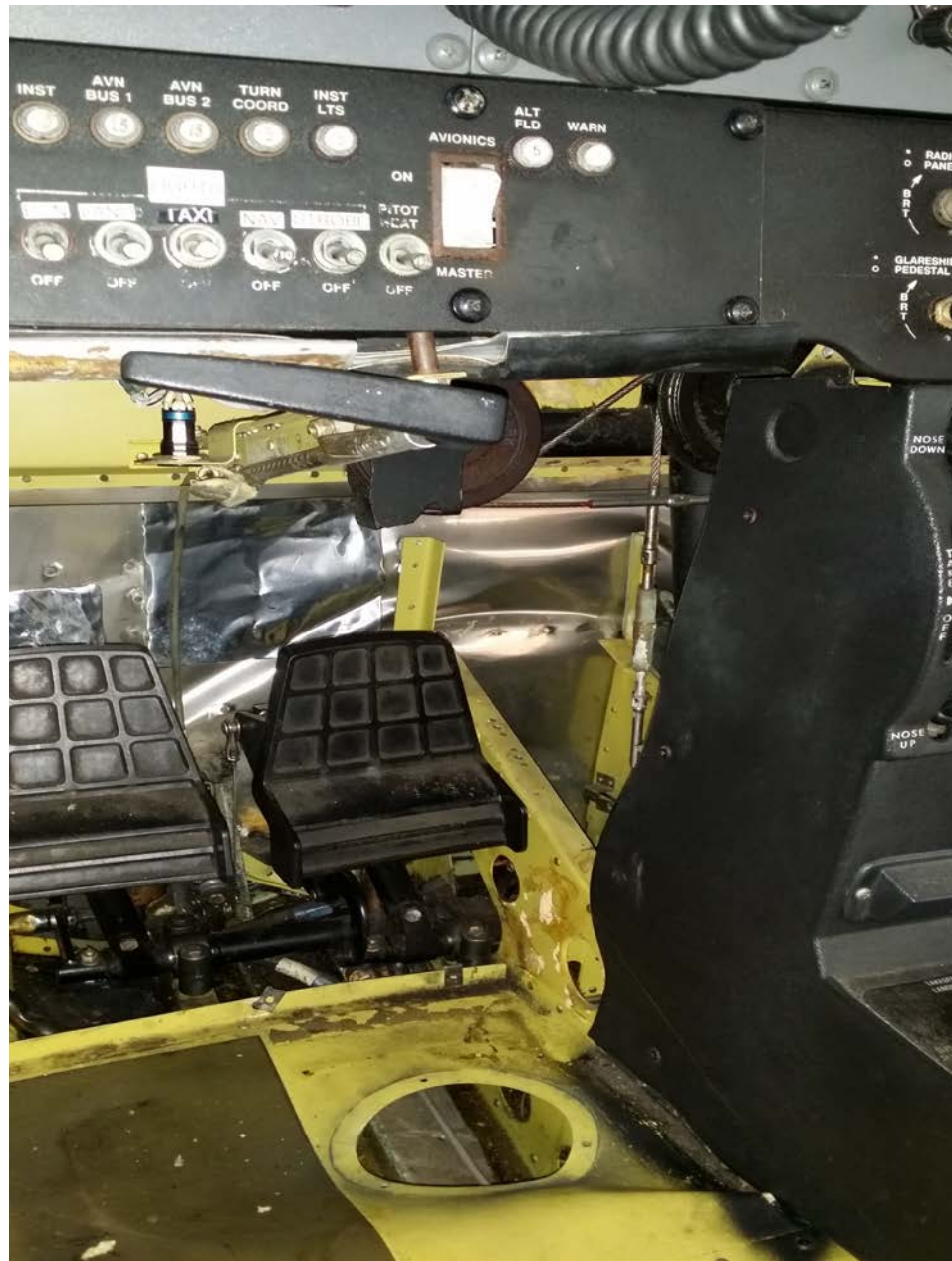
Photo 2 – Interior view of Firewall Damage (Photo Courtesy of FAA)
