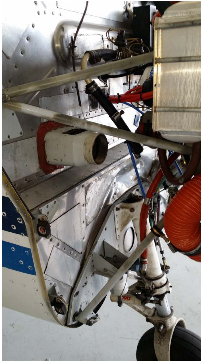
Photo 1 – Substantially Damaged Firewall (Photo Courtesy of FAA)
