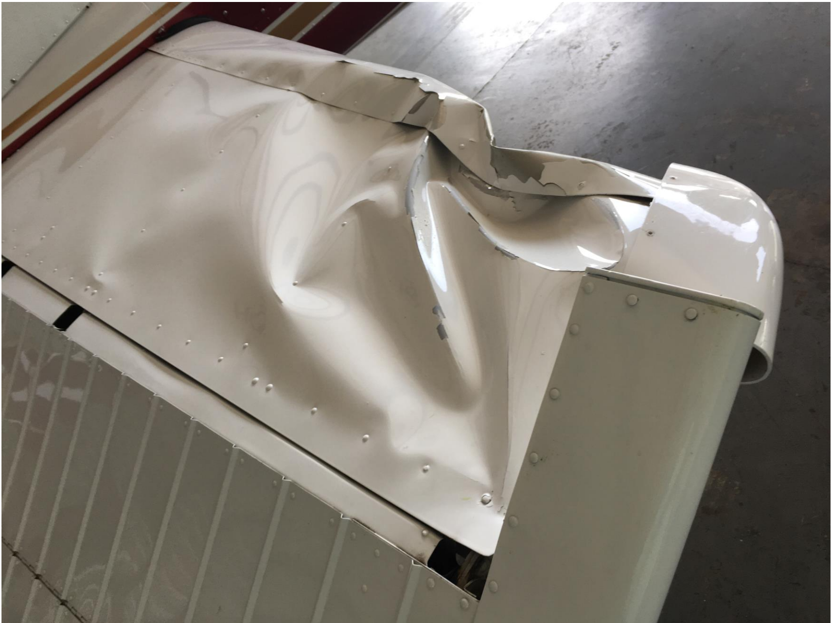
Photo 1 – View of empennage damage. (photo courtesy of the FAA)
