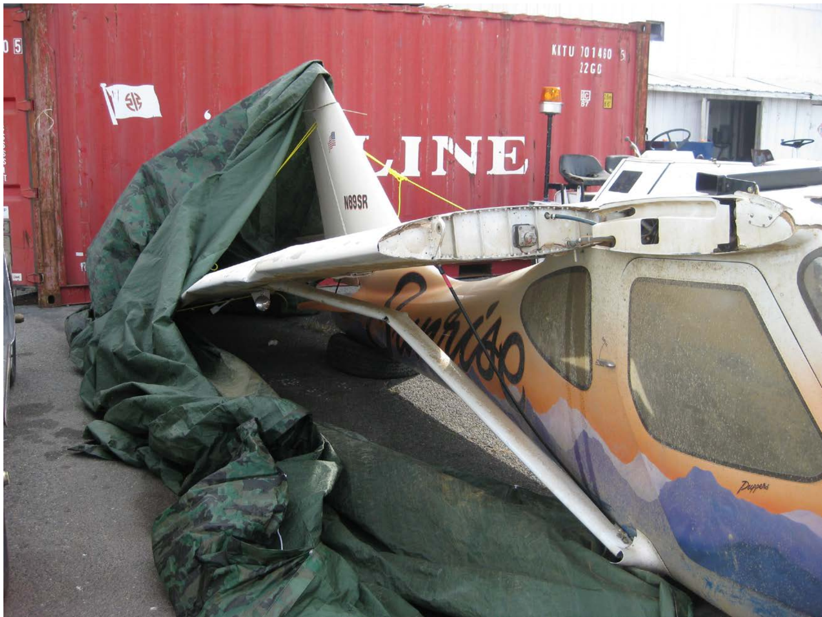
Photo 1 – View of Bent Right Wing Lift Strut (Photo Courtesy of FAA)
