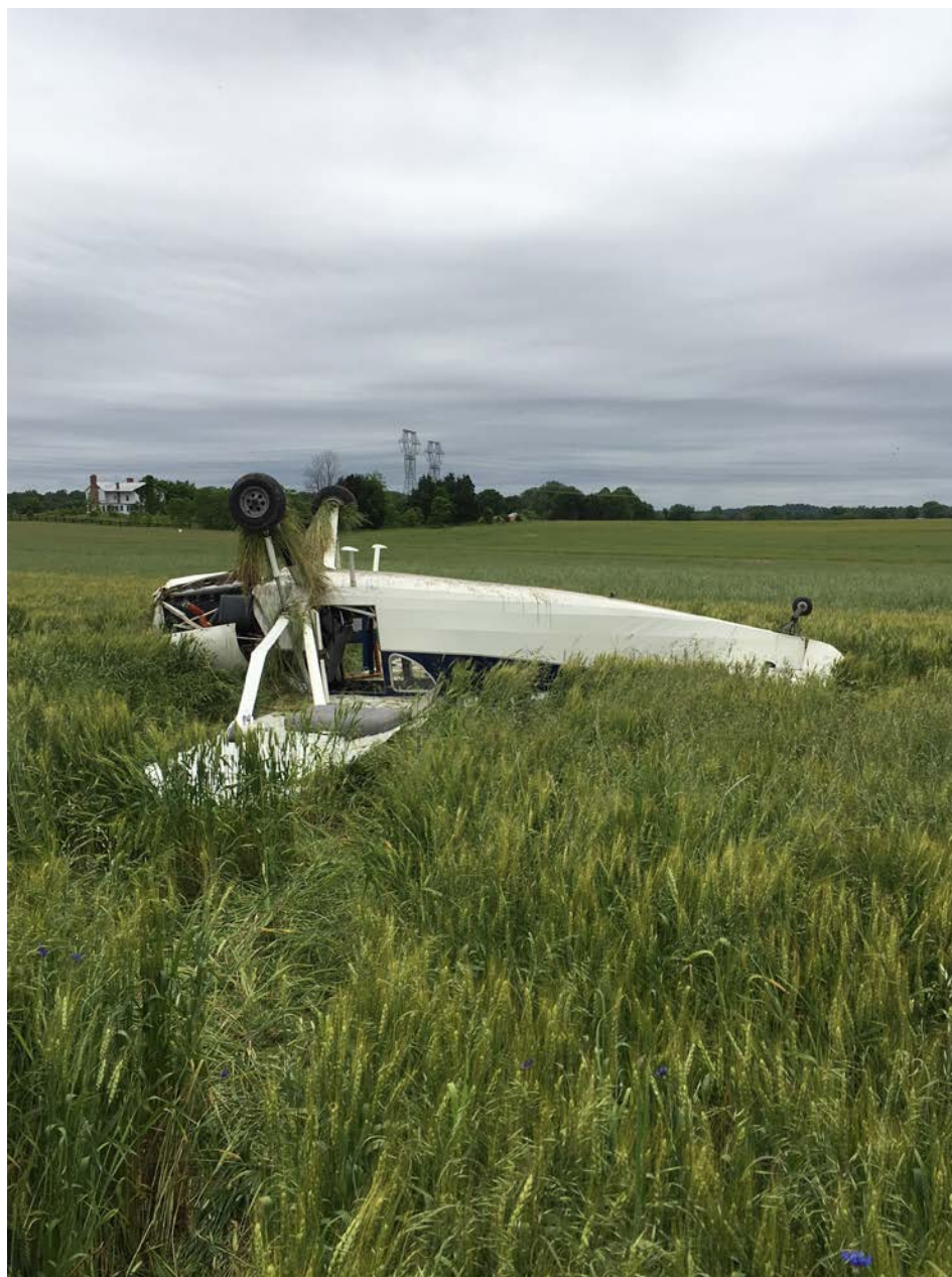
Photo 1 – View of damage to the rudder, the vertical stabilizer and the right wing strut (Courtesy of FAA)
