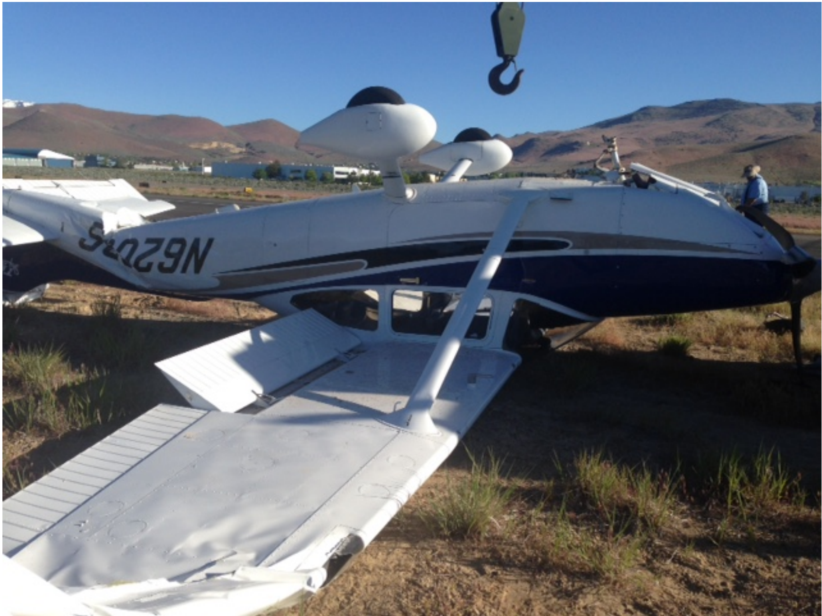
Photo 1 – View of damage to right wing spar and empennage (Courtesy of FAA)
