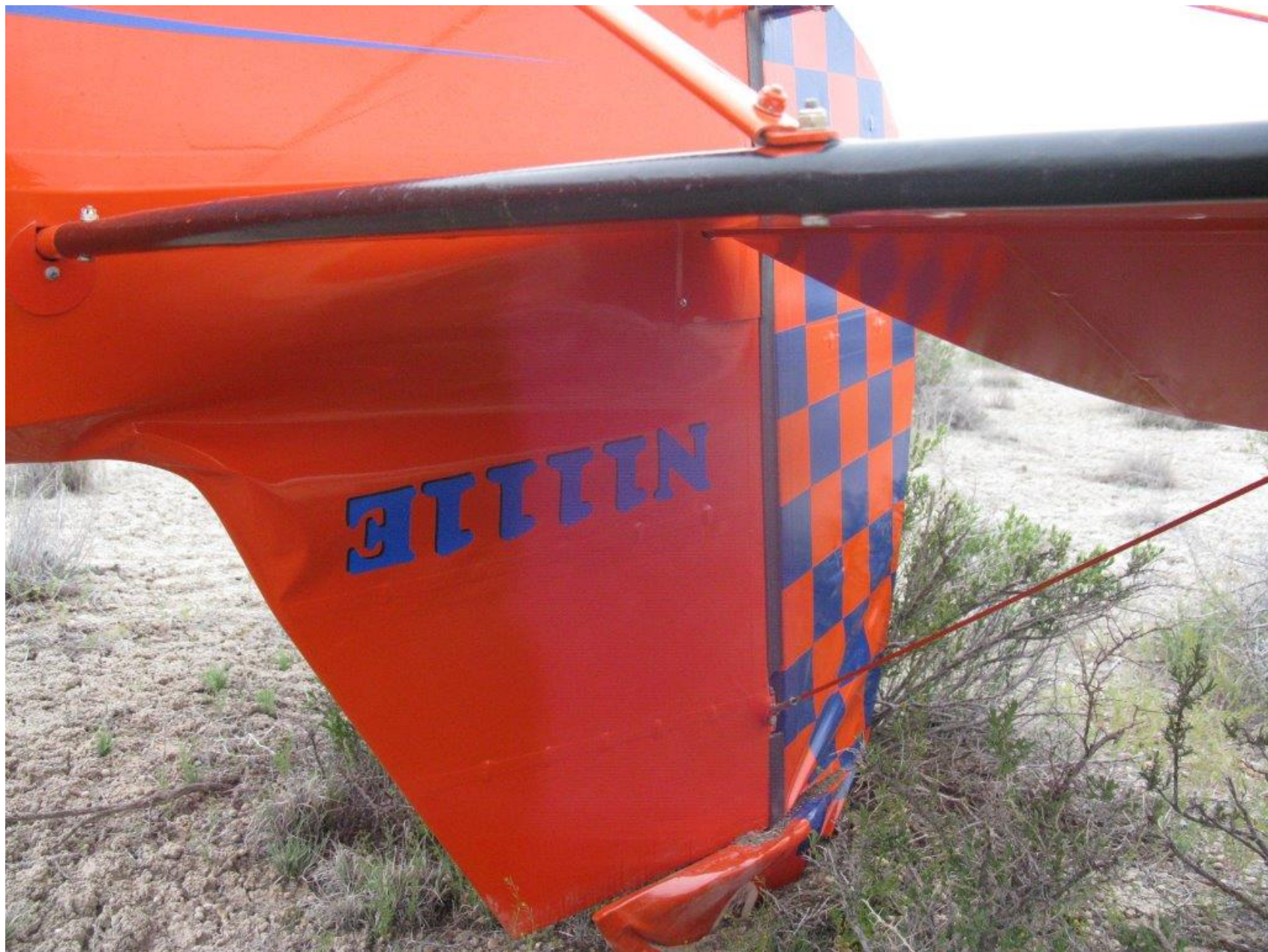
Photo 1 – View of substantial damage to horizontal stabilizer and rudder (Courtesy of FAA)
