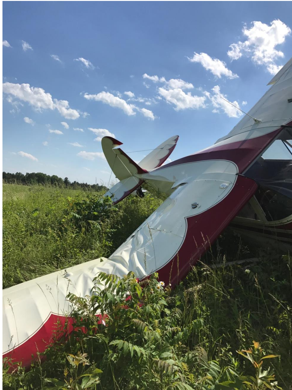
Photo 1 – Front view of damaged right wing (Photo courtesy of the FAA)
