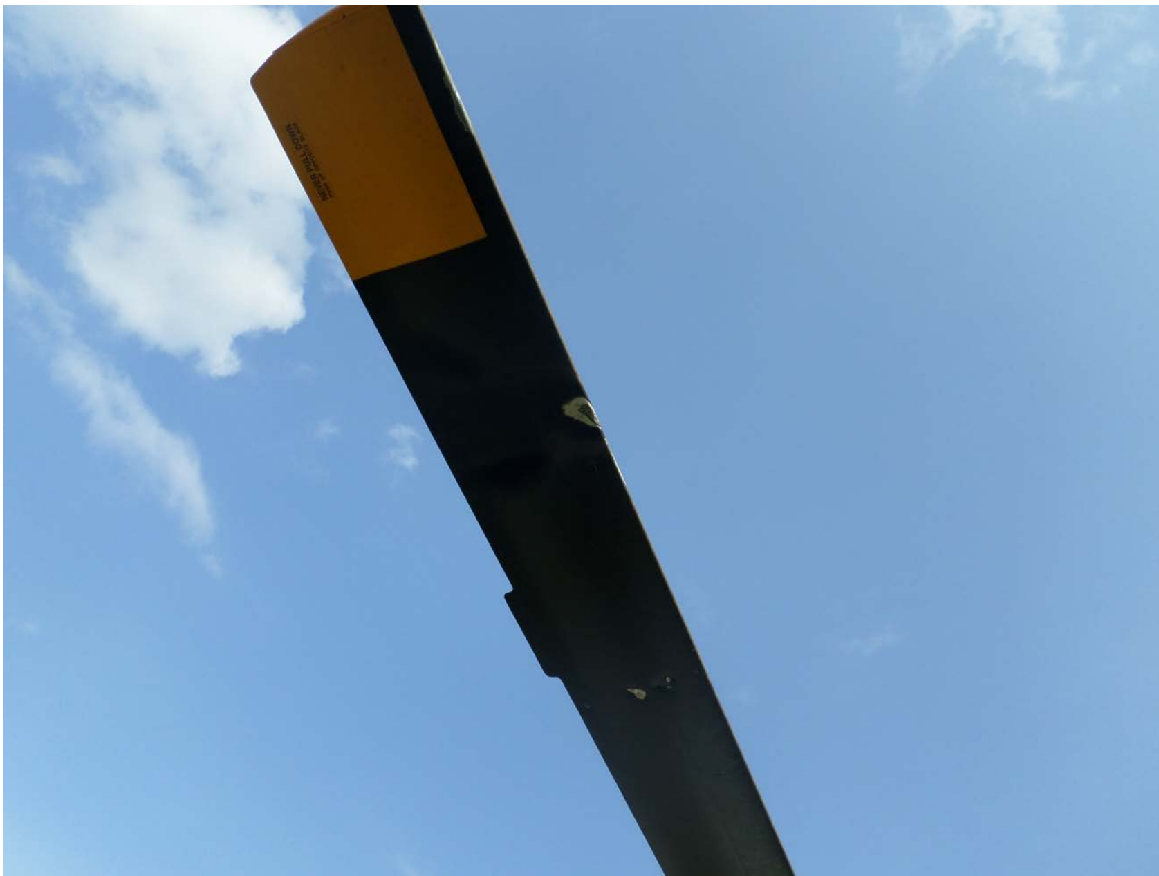
Photo 1 – View of damage to main rotor blade (Courtesy of FAA)
