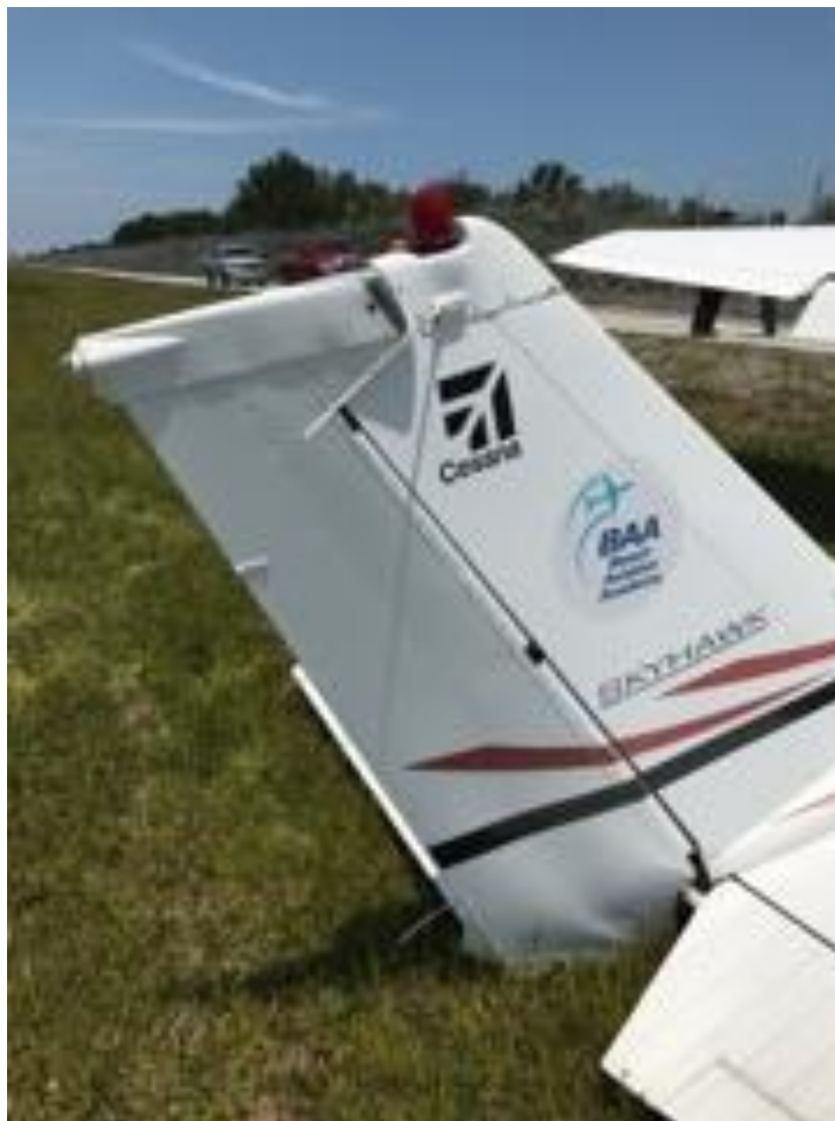
Photo 1 – View of damaged rudder (Photo courtesy of the FAA)
