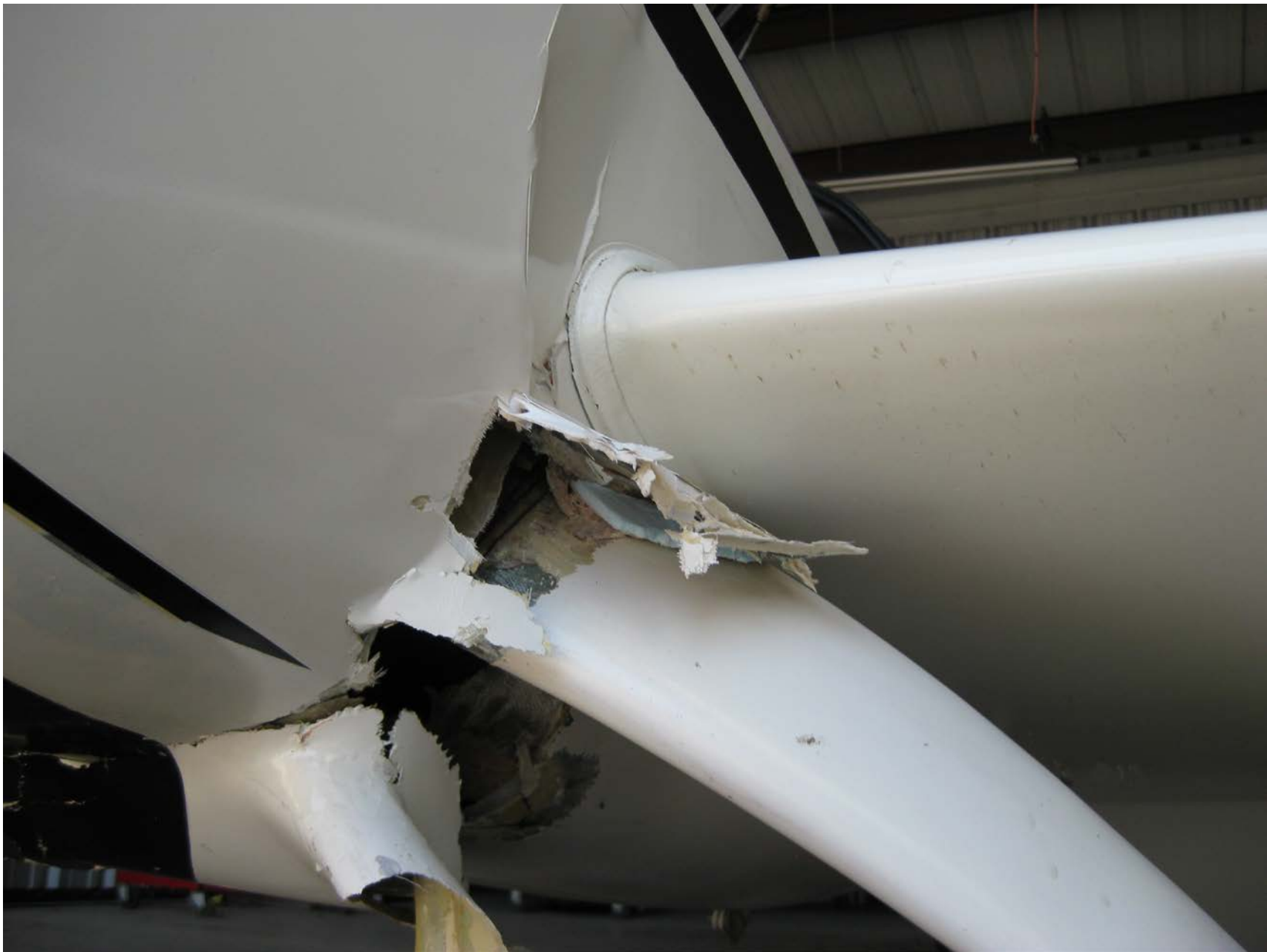
Photo 1 – View of damaged fuselage near left main landing gear (photo courtesy of the FAA)
