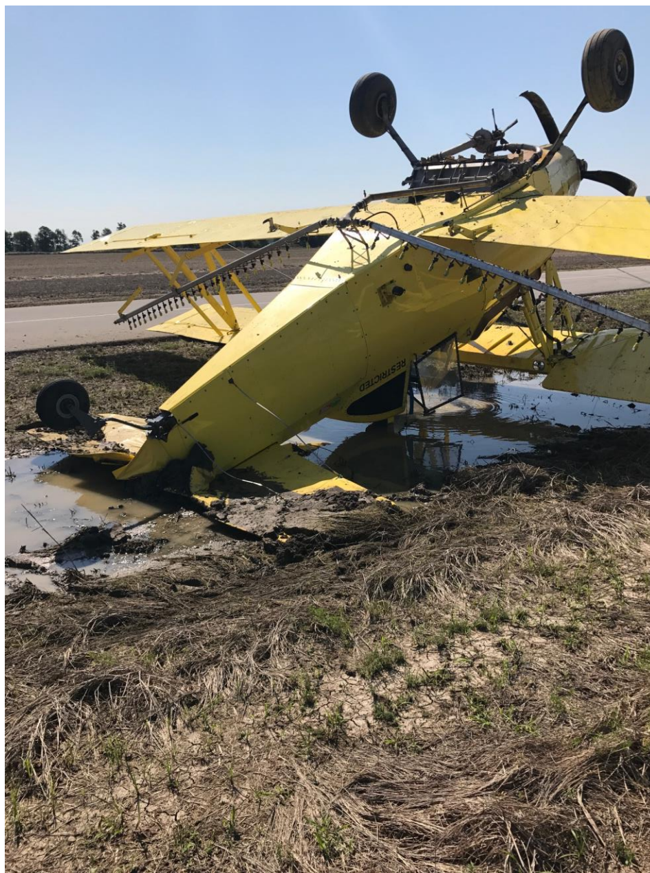
Photo 1 – View of substantial damaged empennage (photo courtesy of the FAA)
