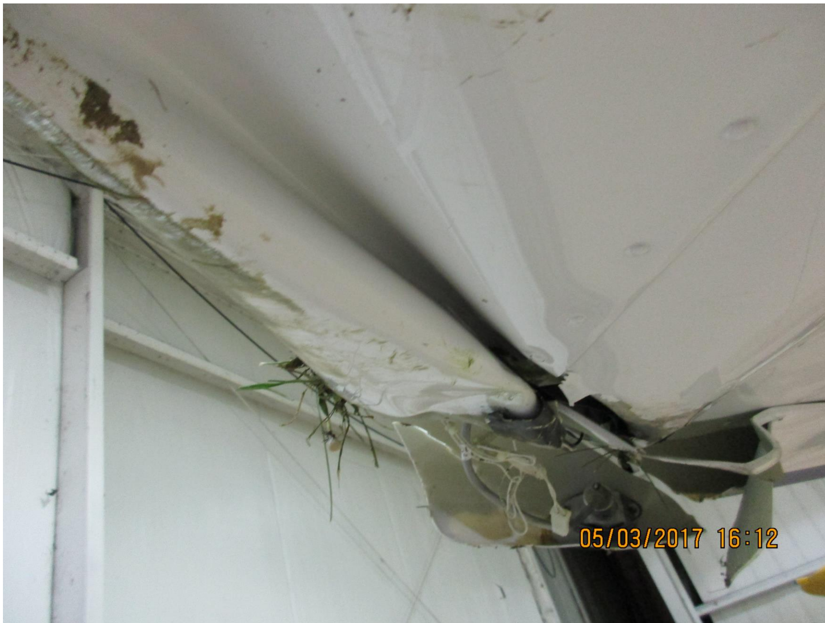
Photo 1 – View of the right wing damage (photo courtesy of the FAA)
