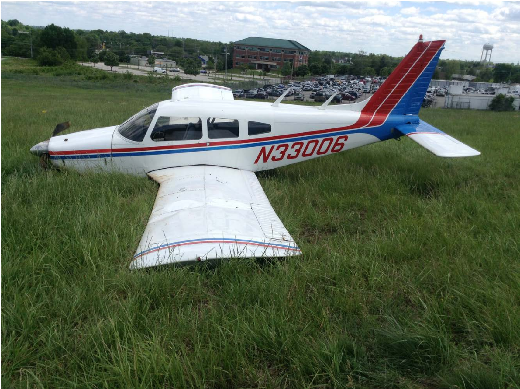
Photo 1 – View of damaged left wing (photo courtesy of the FAA)
