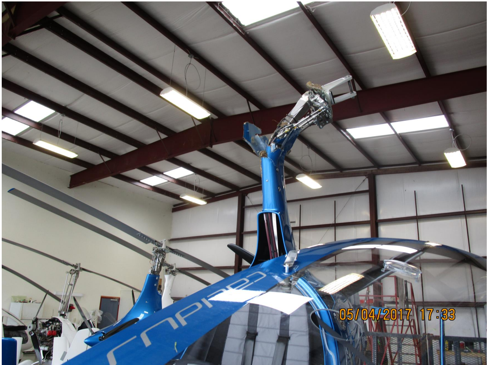
Photo 1 – View of damaged mast beam and rotor (Photo courtesy of the FAA)
