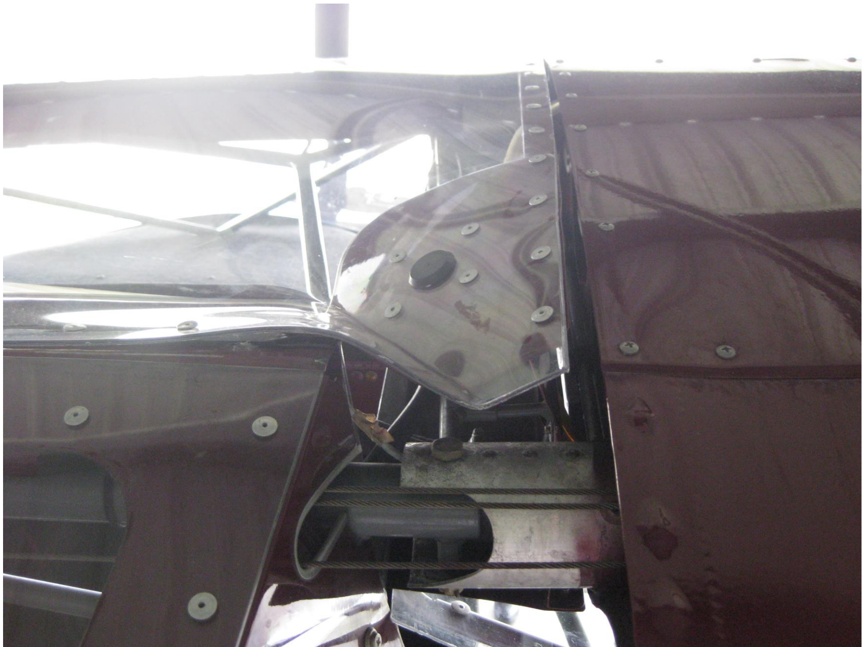
Photo 1 – Rear view of damaged right wing spar (Photo courtesy of the FAA)
