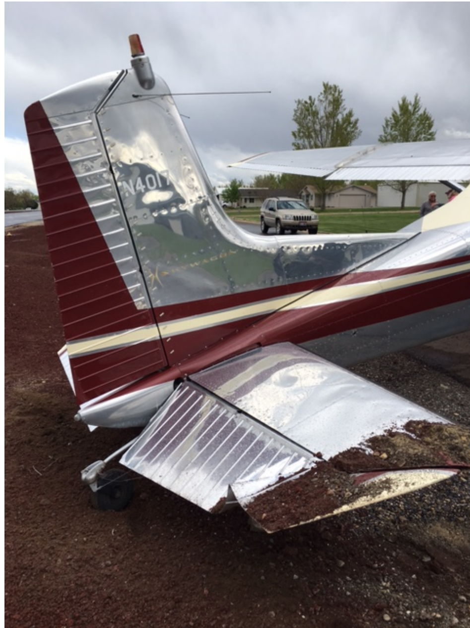
Photo 1 – View of damage to the right elevator (Courtesy of FAA)
