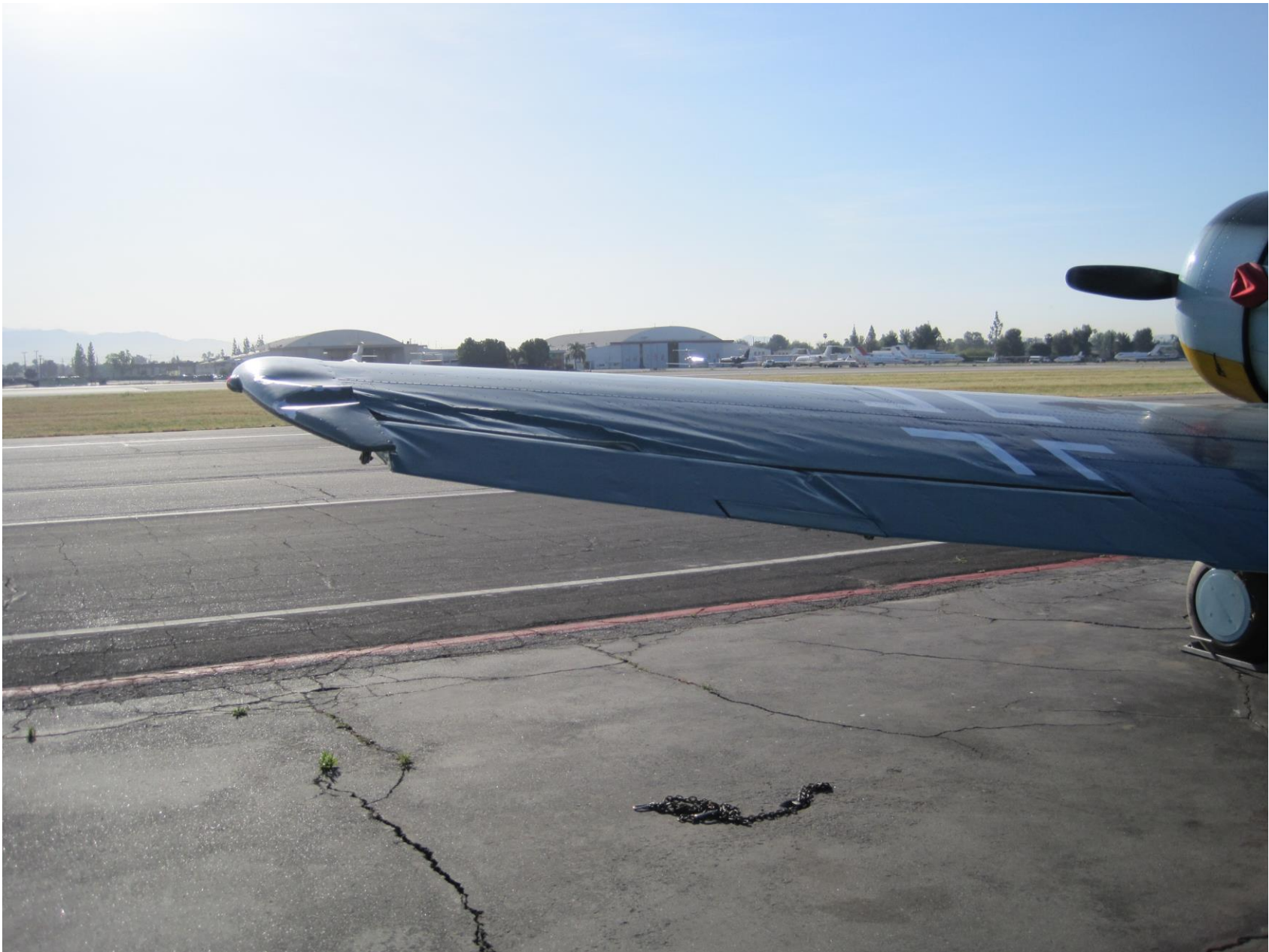
Photo 1 – Rear view of damaged left wing and aileron (Photo courtesy of the FAA)
