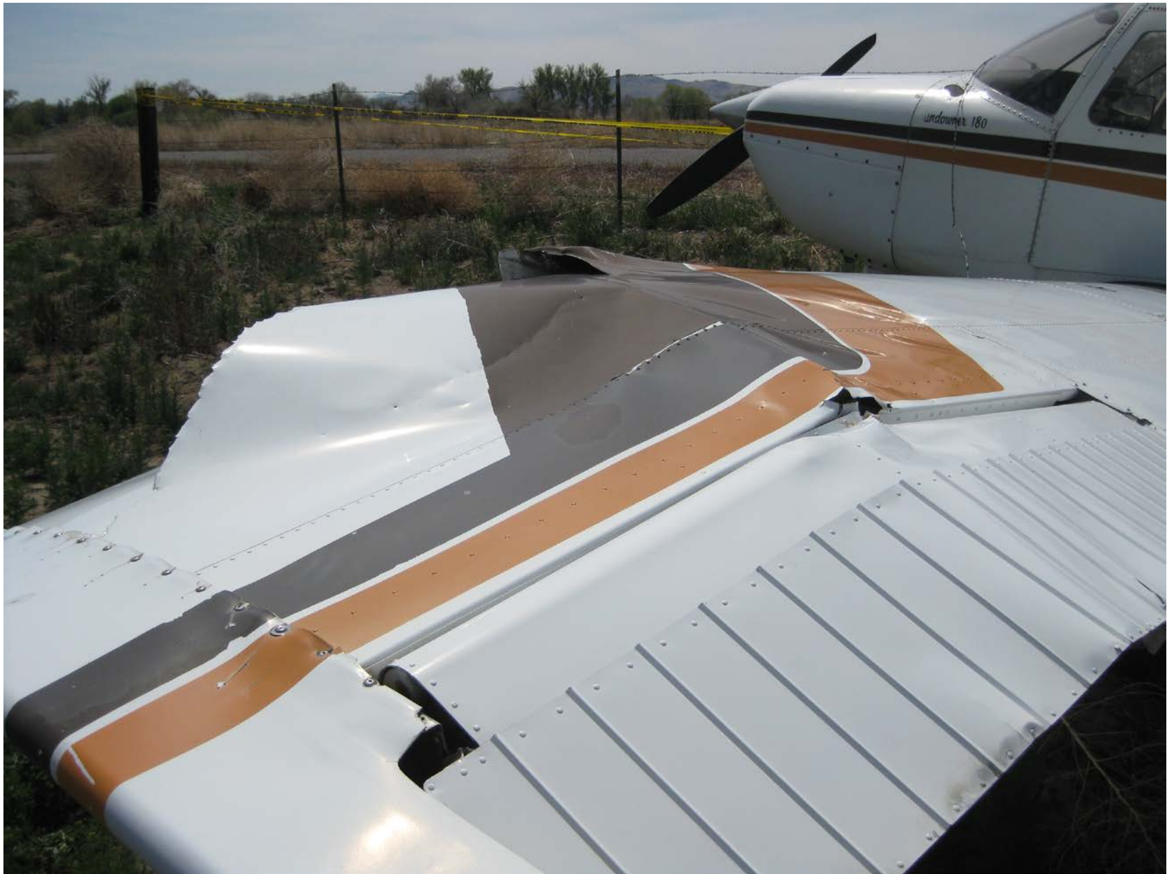
Photo 2 – Substantial Damage to Left Wing (Photo Courtesy of FAA)
