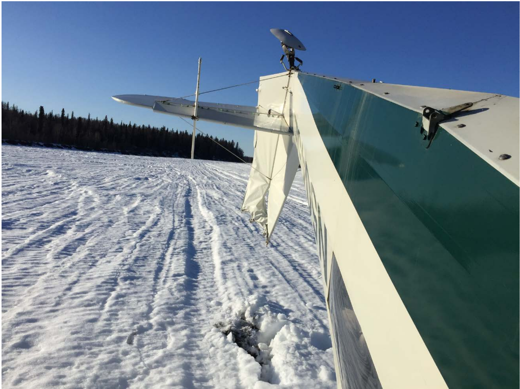
Photo 2 – Substantially Damaged Vertical Stabilizer (Photo Courtesy of Operator)
