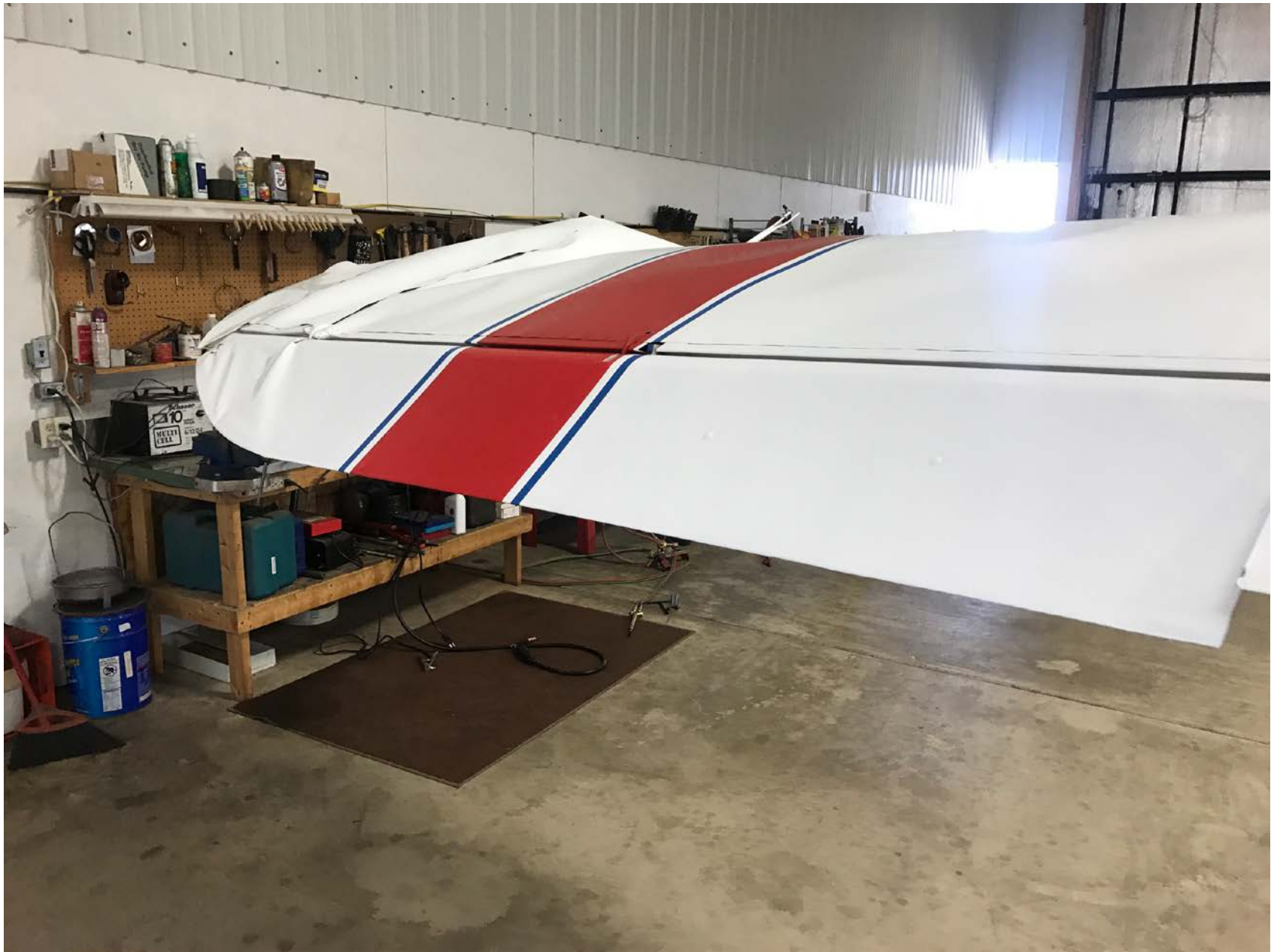
Photo 2 – Substantial Damage to the Left Wing (Photo Courtesy of FAA)
