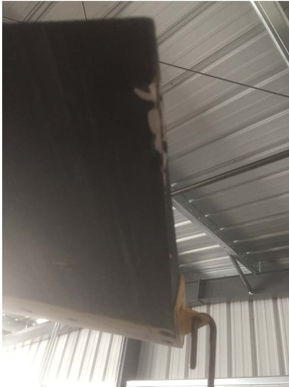
Photo 2 – View of damage to main rotor blade (Courtesy of FAA)
