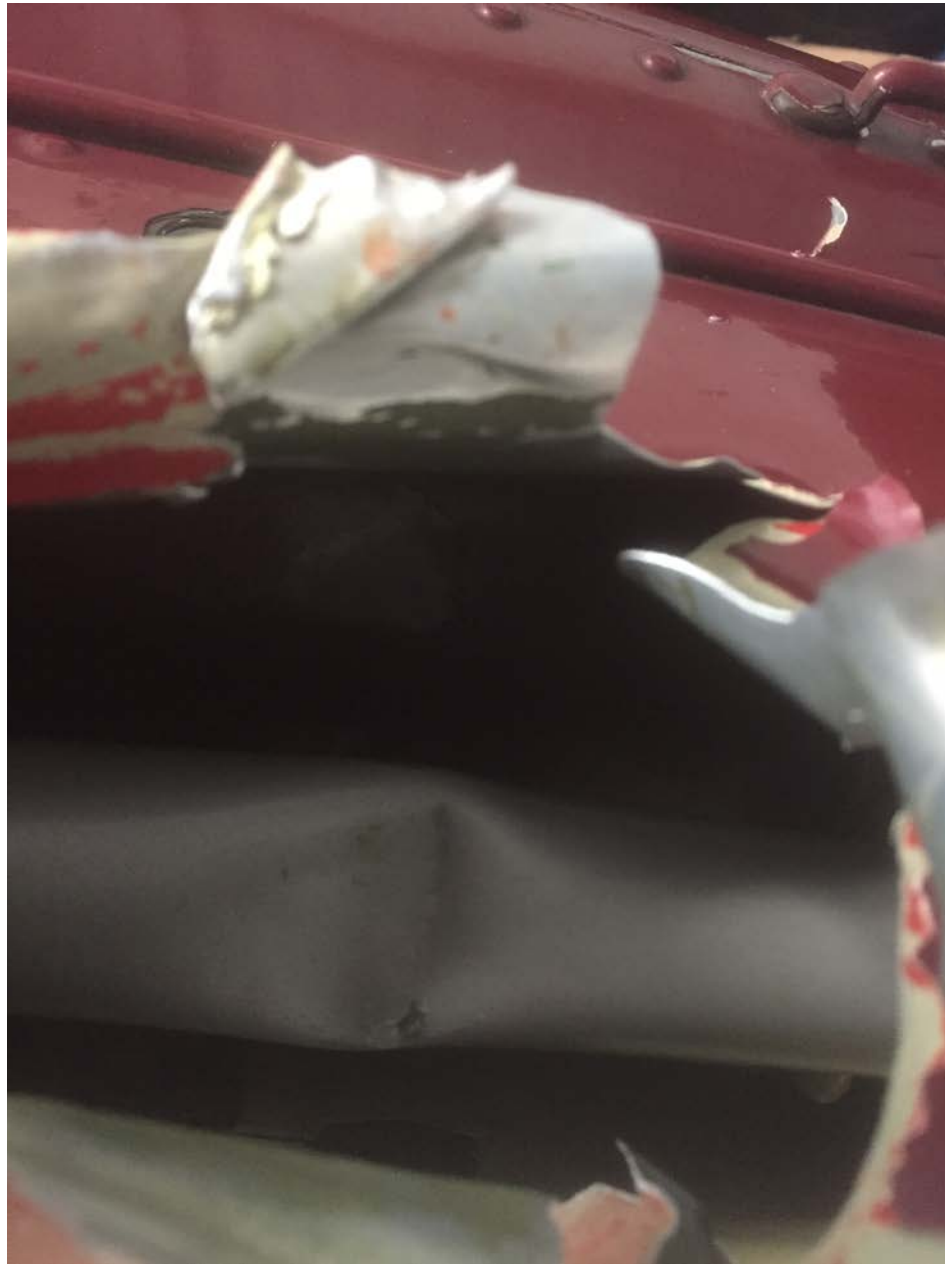
Photo 1 – View of damage to tail rotor driveshaft (Courtesy of FAA)
