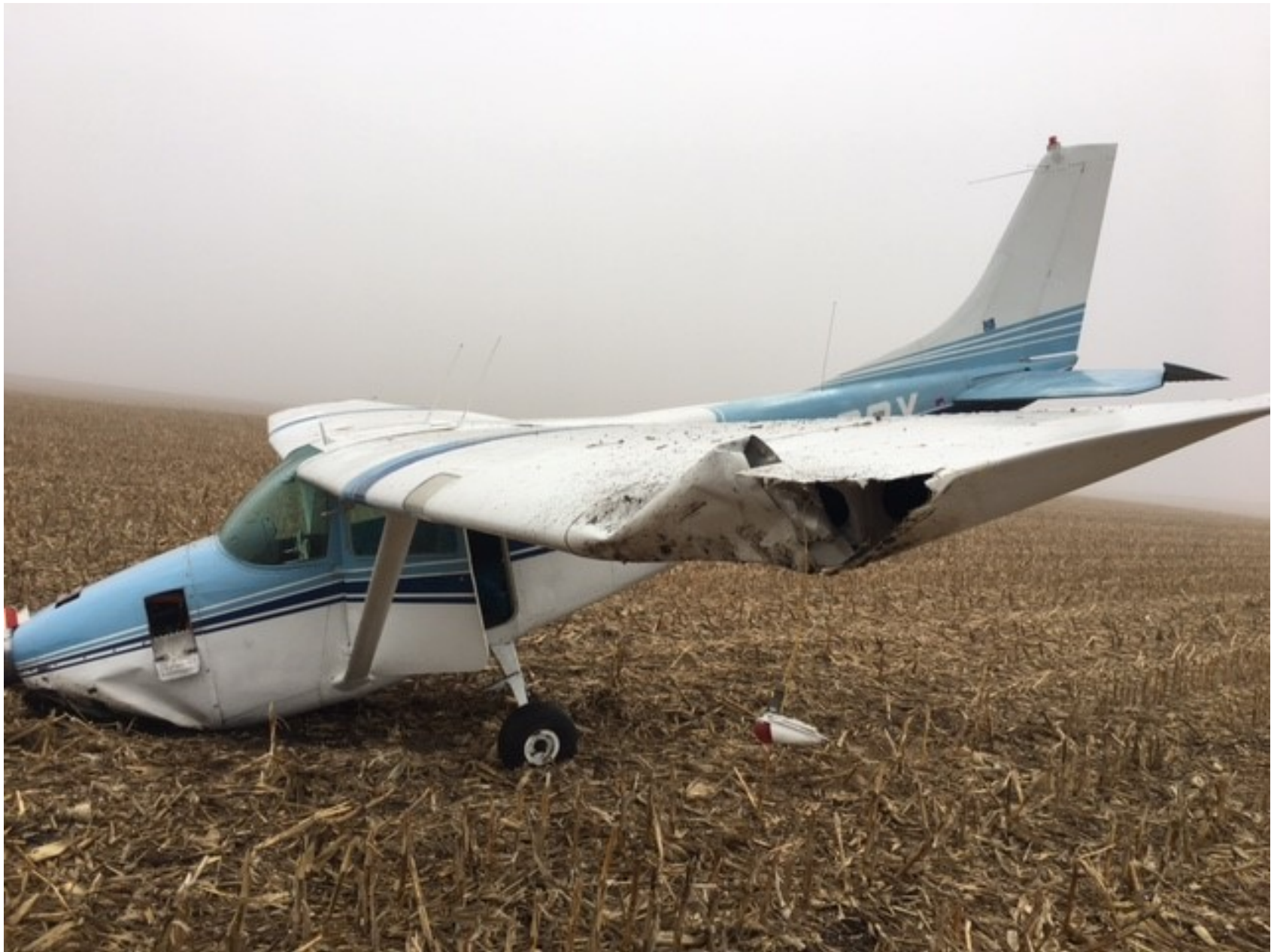
Photo 1 – View of Airplane with Collapsed Nose Gear in a Field (Photo Courtesy of FAA)
