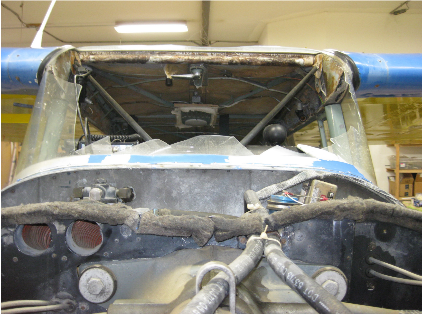
Photo 2 – View of damaged windshield (photo courtesy of the FAA)
