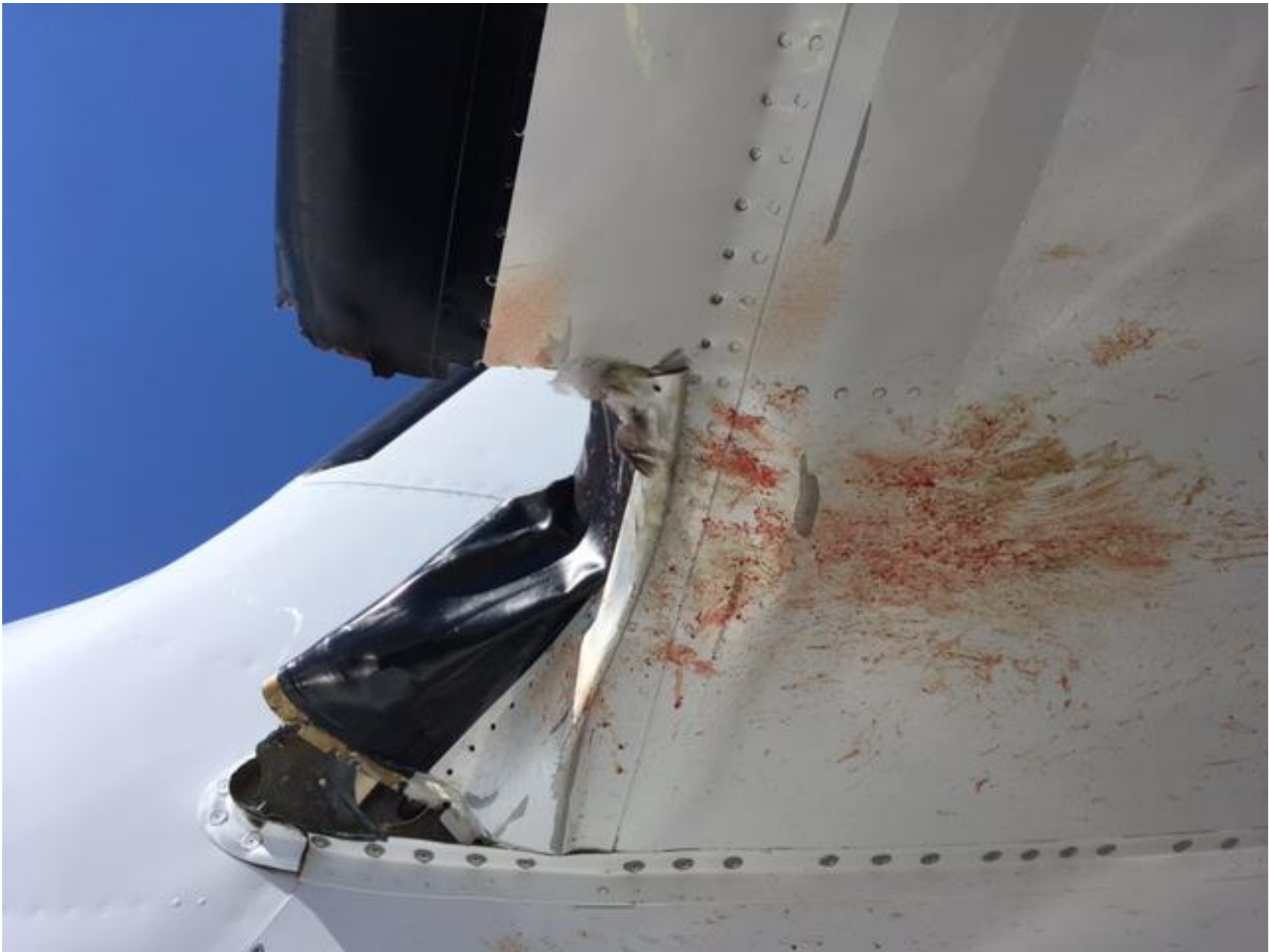
Photo 1 – View of bird strike on left horizontal stabilizer (Photo courtesy of the FAA)
