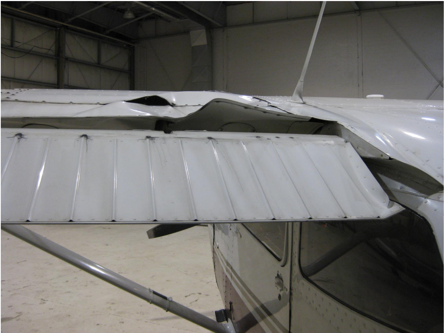
Photo 1 – View of the left wing damage (photo courtesy of the FAA)
