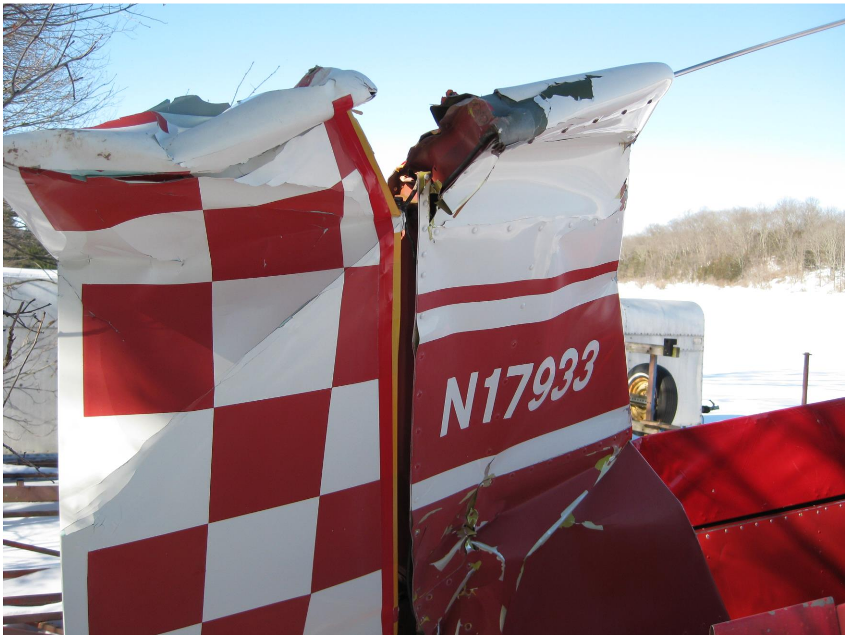
Photo 1 – View of damaged rudder (Photo courtesy of the FAA)
