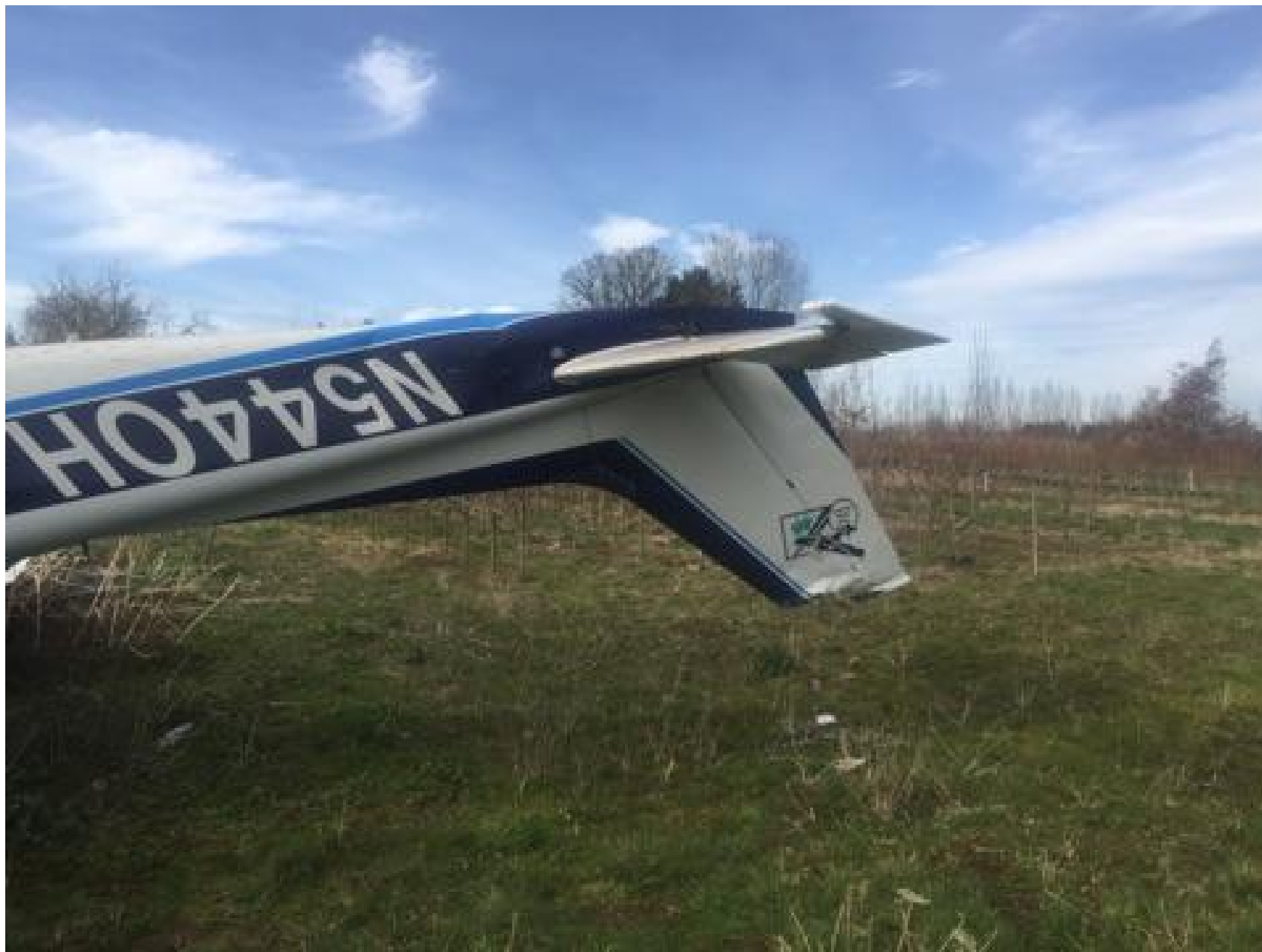
Photo 2 – Substantially Damaged Vertical Stabilizer (Photo Courtesy of FAA)
