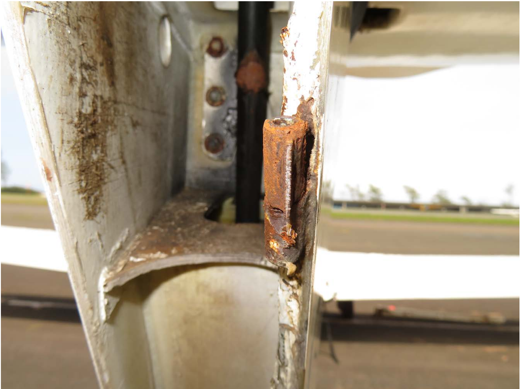
Photo 3 – View of upper rudder attachment hinge (photo courtesy of the FAA)
