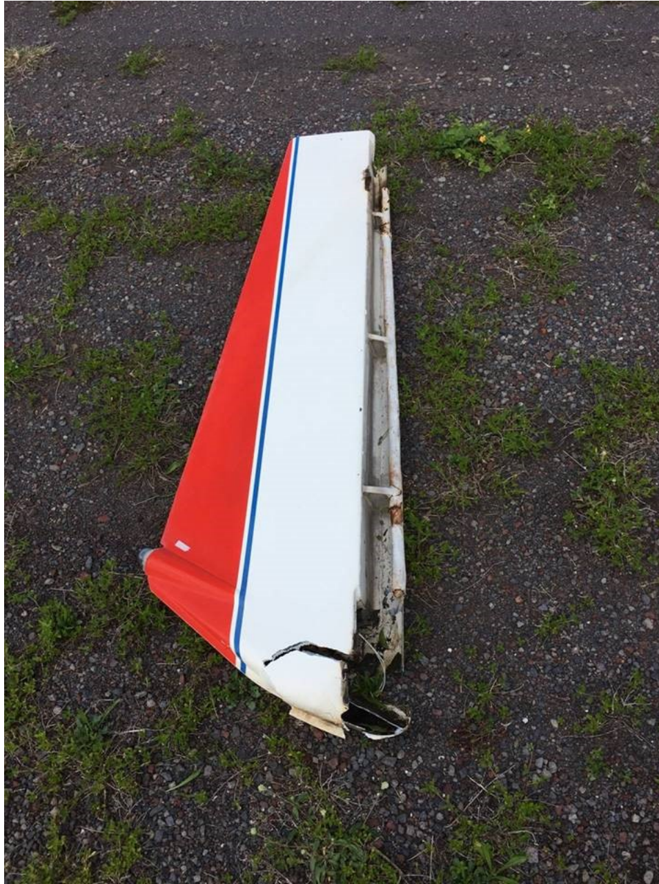
Photo 2 – View of separated rudder (photo courtesy of the pilot)
