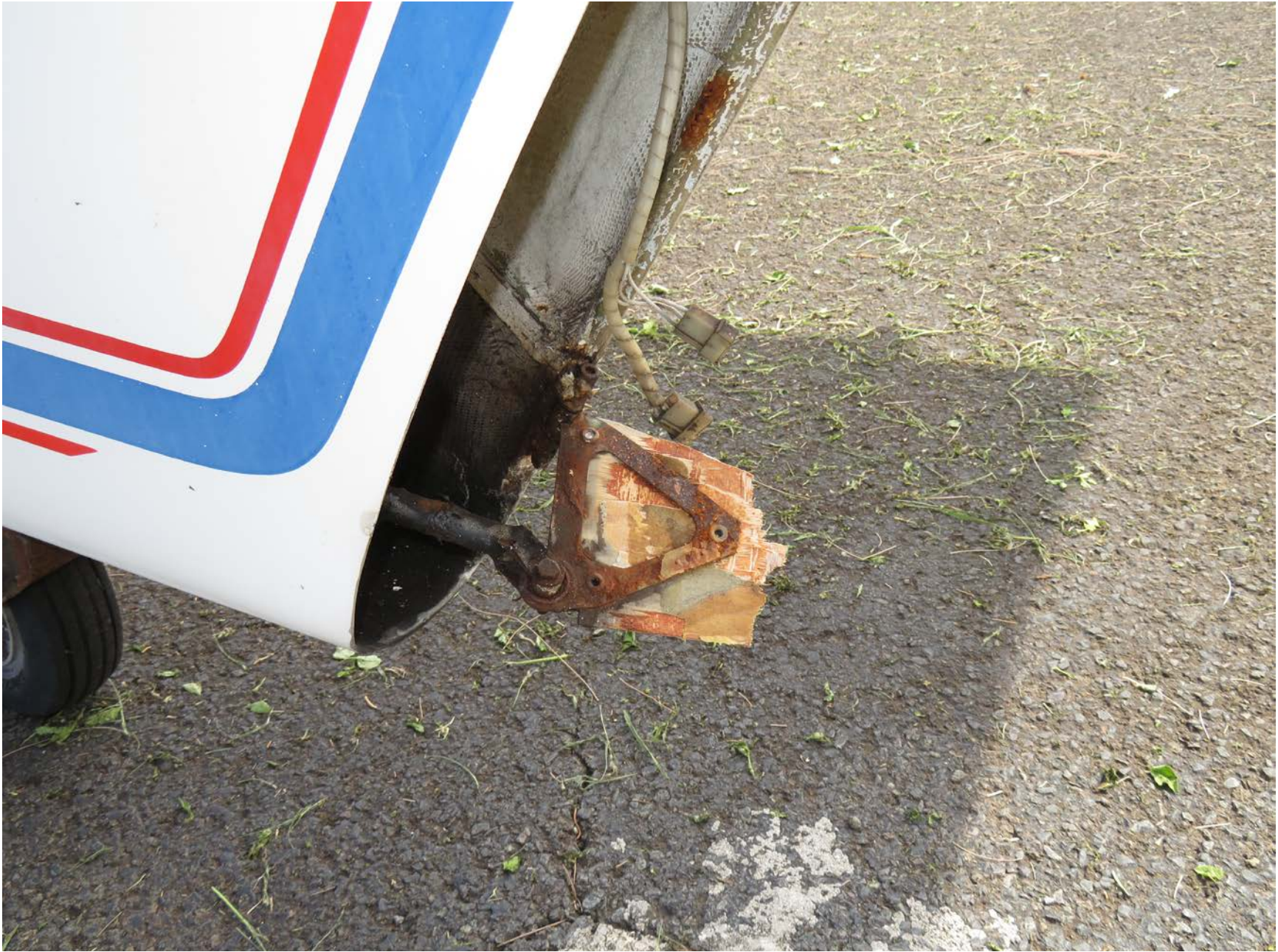
Photo 4 – View of lower rudder attachment hinge (photo courtesy of the FAA)
