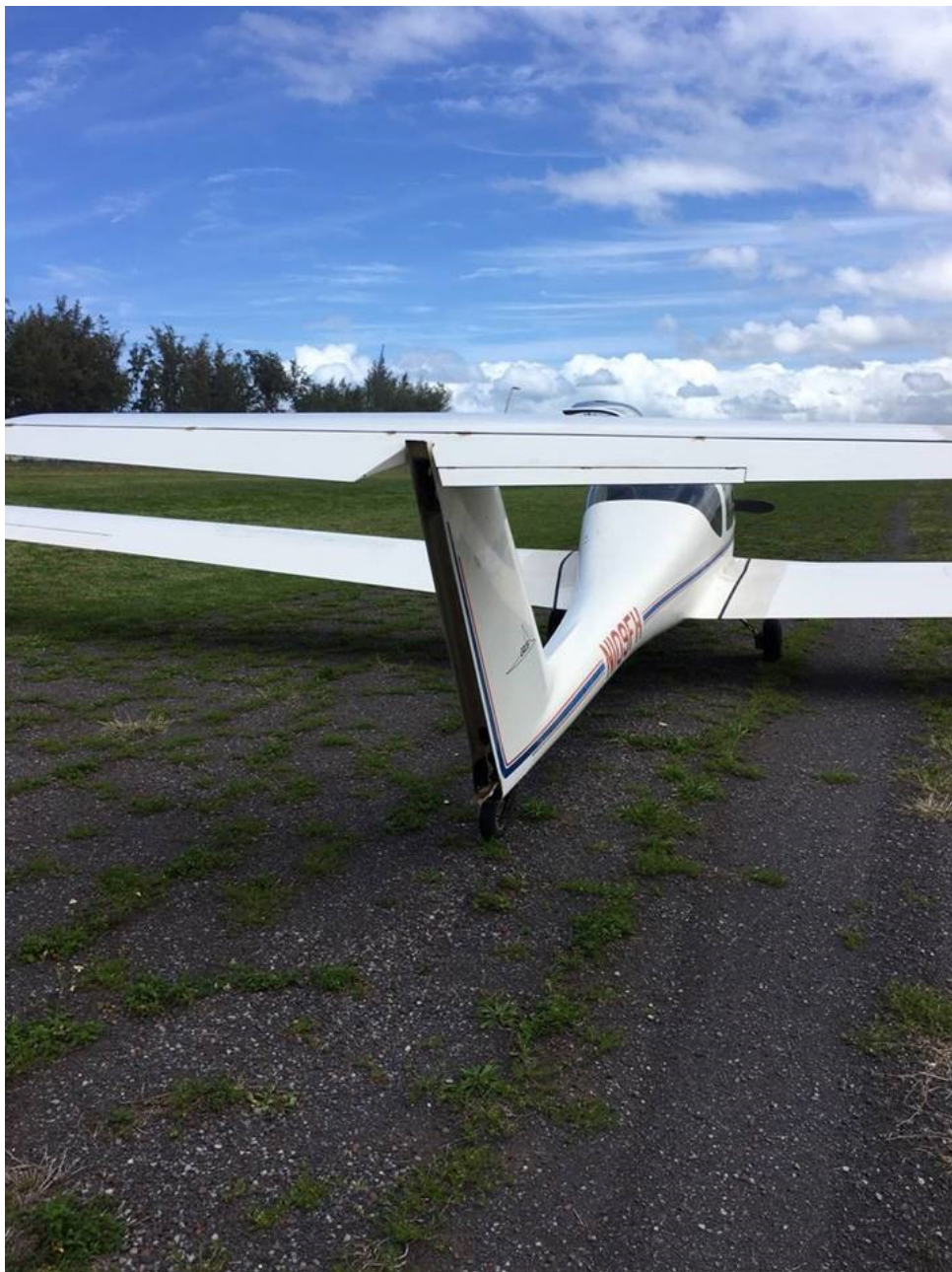
Photo 1 – View of powered glider from rear without rudder (photo courtesy of the pilot)
