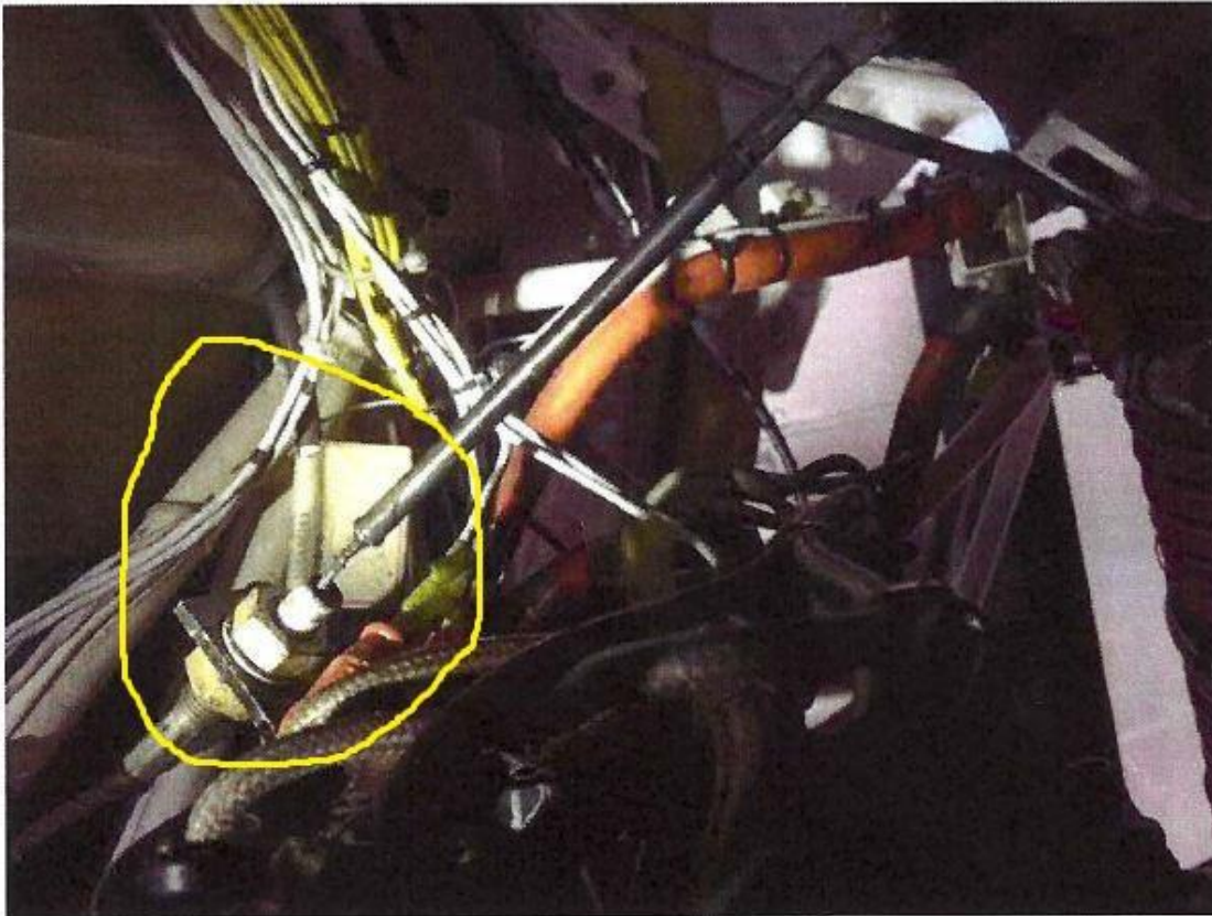
Throttle cable at full throttle
