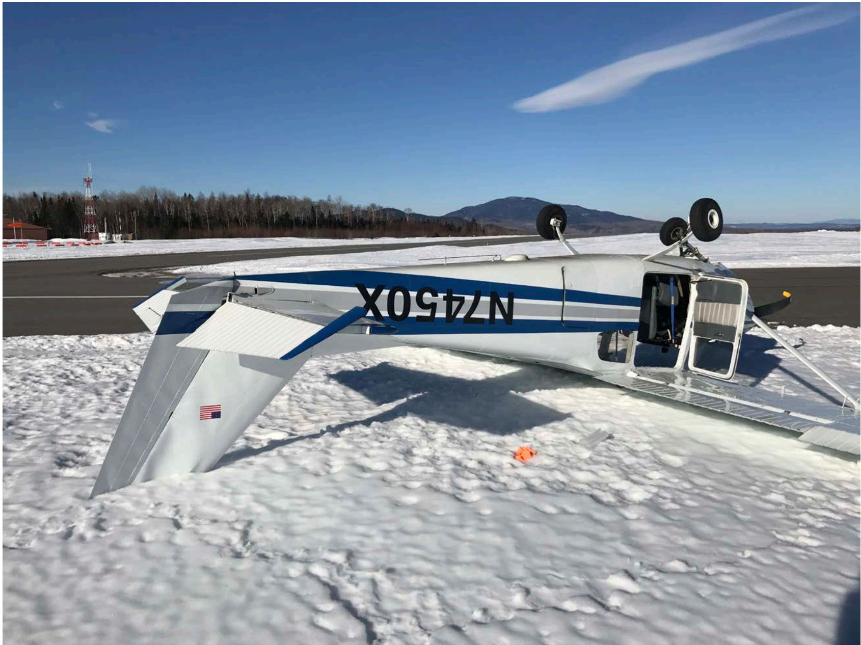
Photo 1 – Substantially Damaged Vertical Stabilizer (Photo Courtesy of FAA)
