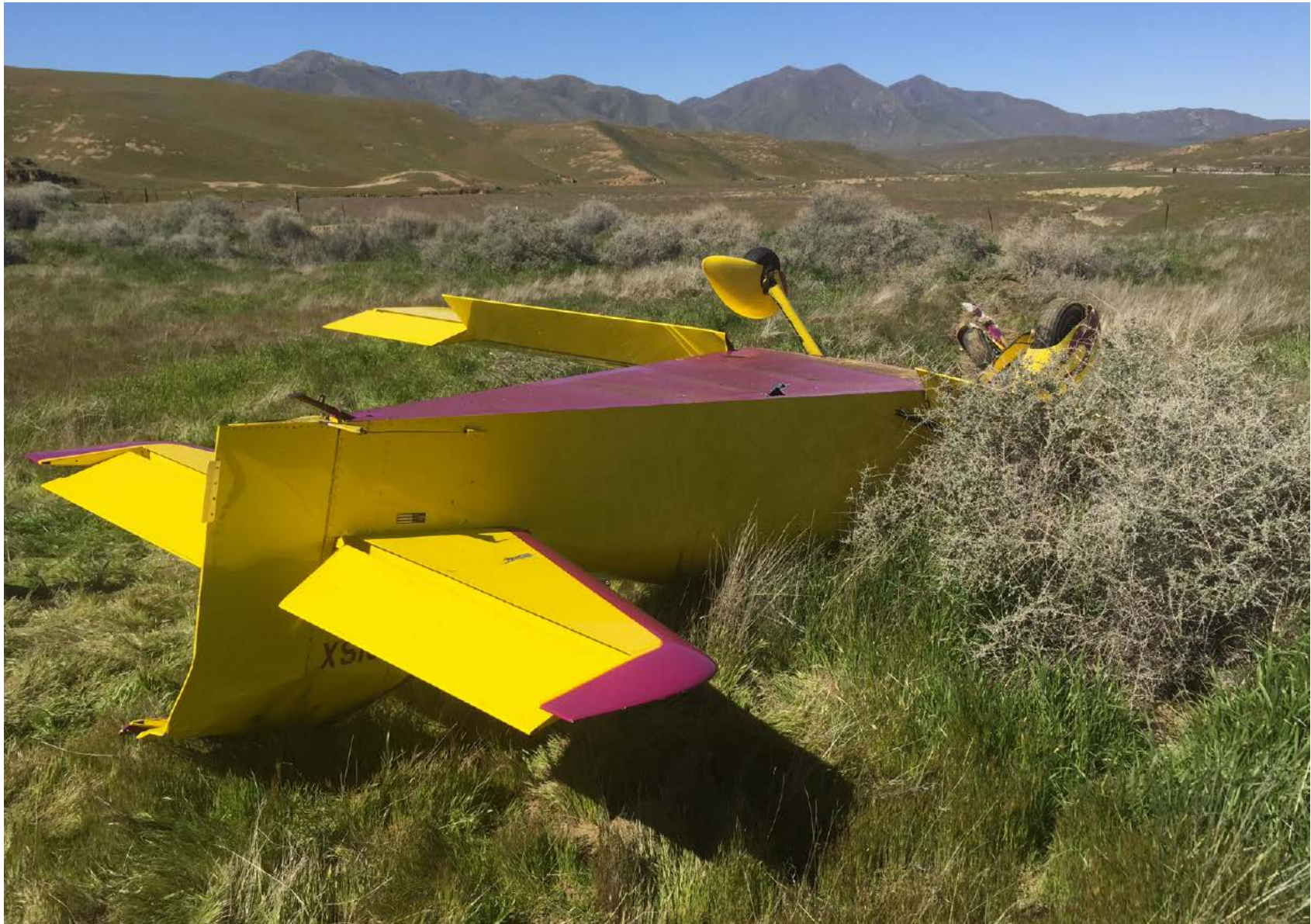
Photo 1 – View of damage to vertical stabilizer and rudder (Courtesy of FAA)
