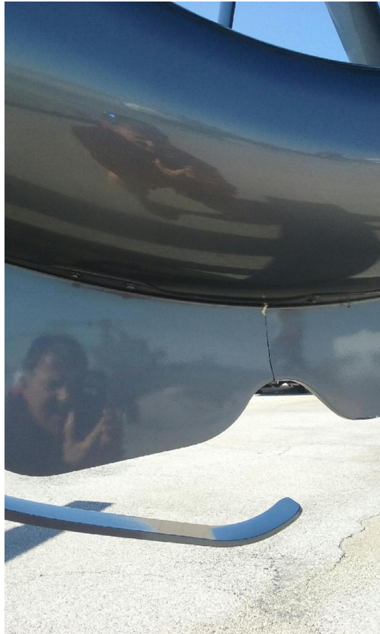
Photo 1 – Substantially damaged Fenestron (Photo Courtesy of FAA)
