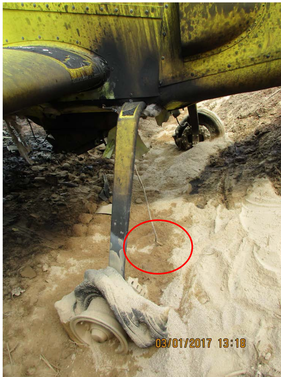
Photo 3 – Separated Hydraulic Brake Line (Photo Courtesy of FAA)
