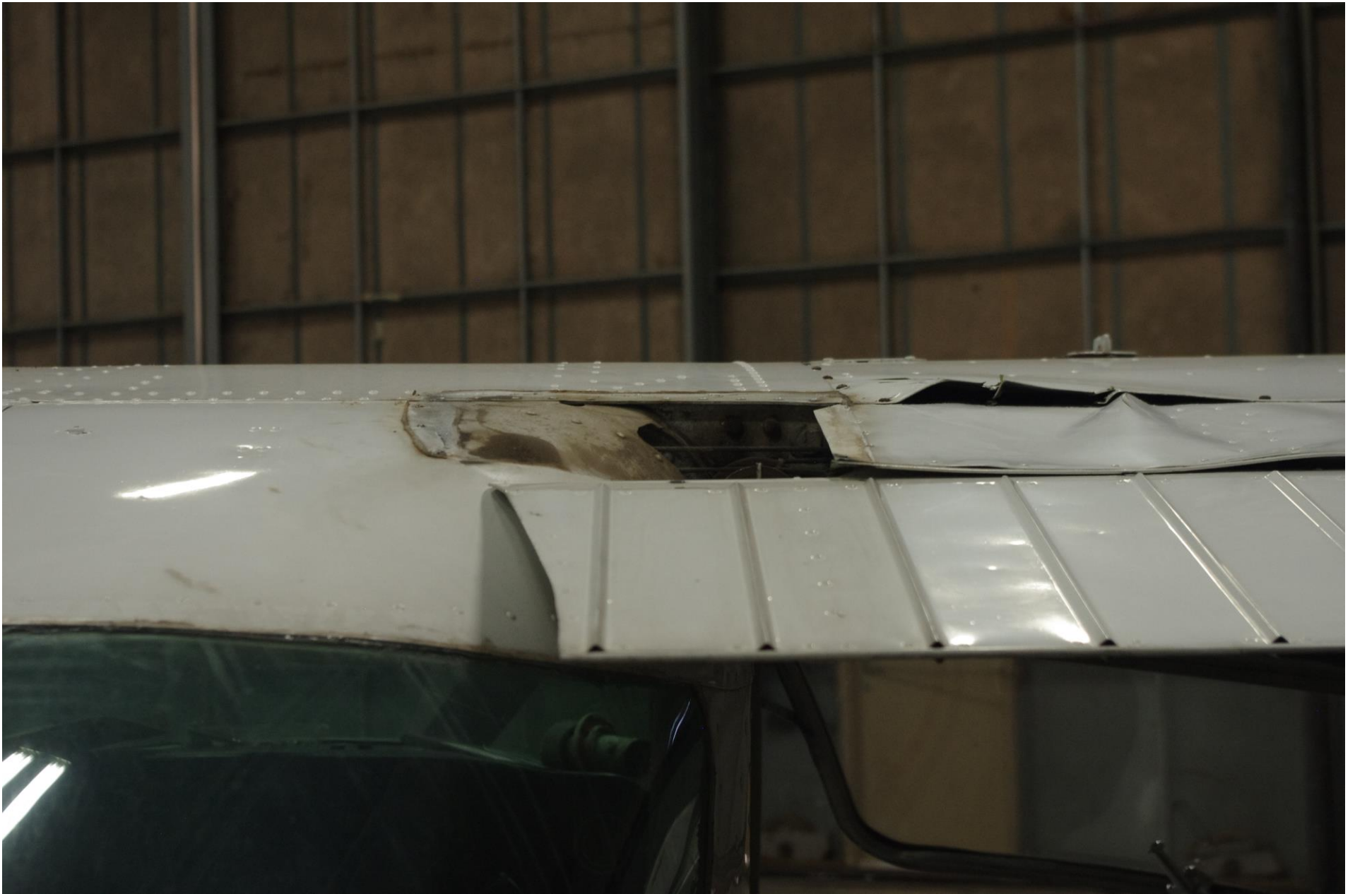
Photo 1 – Rear view of damaged right rear spar (Photo courtesy of the FAA)
