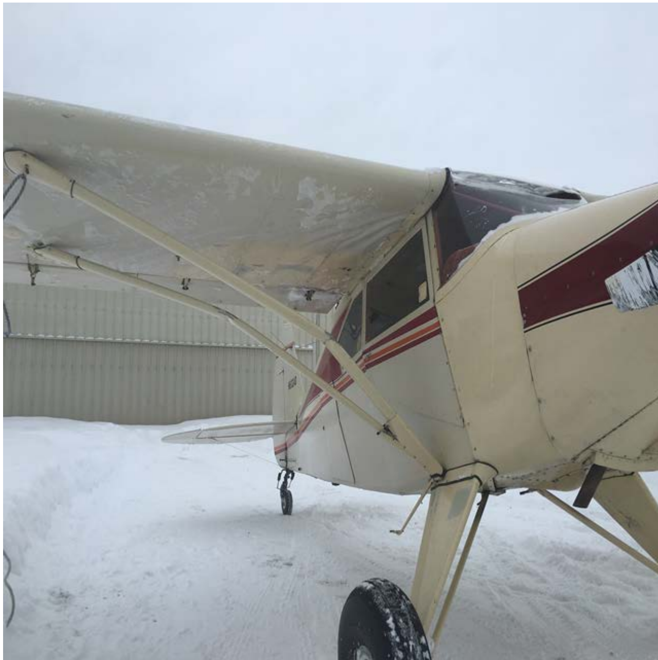
Photo 1 – View of damaged right wing lift strut (photo courtesy of pilot)
