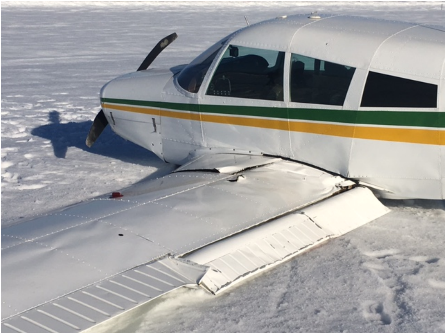
Photo 1 – View of the damage to the left wing (Courtesy of FAA)
